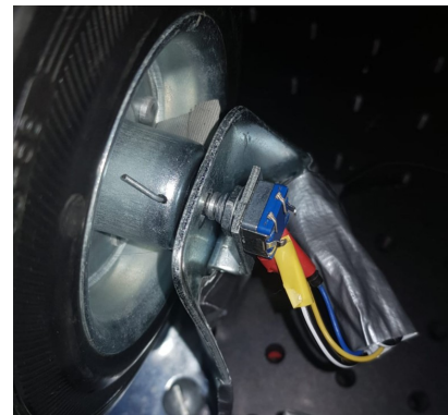
Fig. 9: Rotary encoder attached to wheel axle
