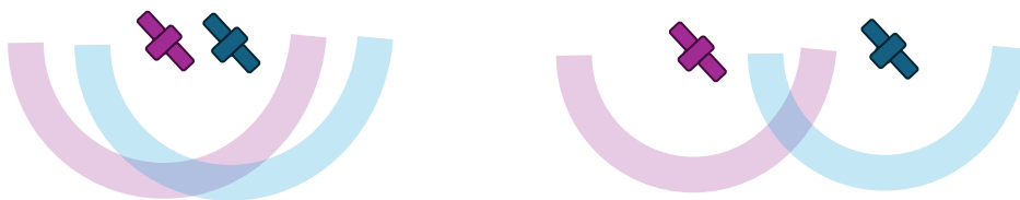
Figure 3.1: 2D representation of Dilution of Precision (DOP) for different relative satellite geometries, where the strips indicate the uncertainty in range to a specific satellite. A smaller overlap area of these strips corresponds to a lower DOP and a lower uncertainty in user position.
