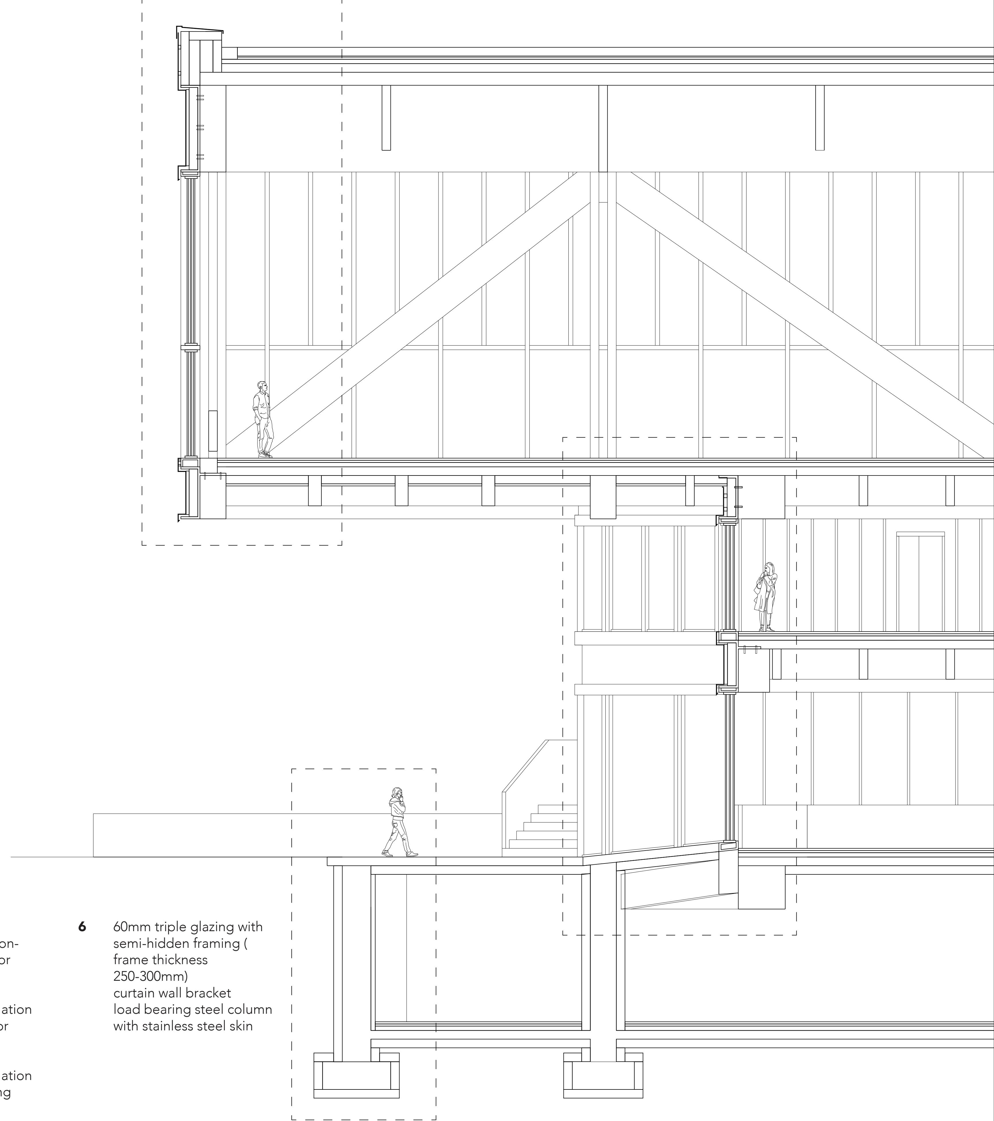
3 100 mm reinforced concrete finishing 50mm light weight concrete screed with floor heating 100mm concrete floor slab 200mm thermal insulation 50mm ceiling finishing
