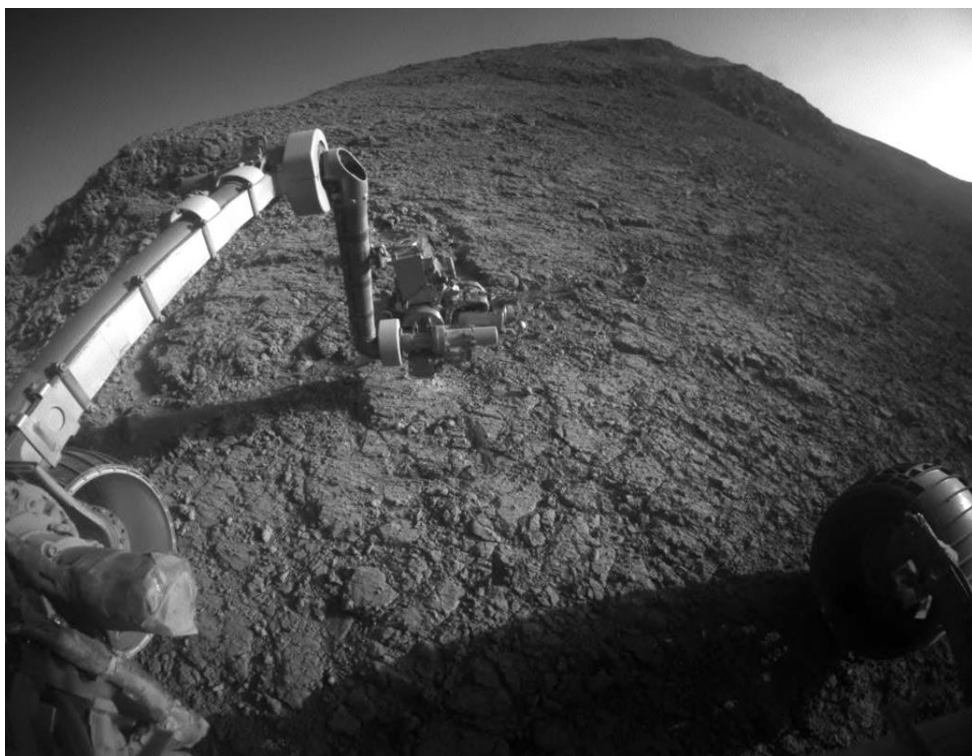
Figure 3. Photograph showing the MIMOS II Mössbauer instrument (pointing towards the sky) attached to the robotic arm of NASA's Opportunity Mars Rover taken on the western rim of Endeavour Crater, Mars (image reprinted from NASA).
