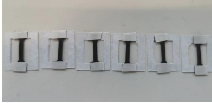
Figure 20. POMaC/CIP samples bonded on the paper frame which is made by blade cutter.
