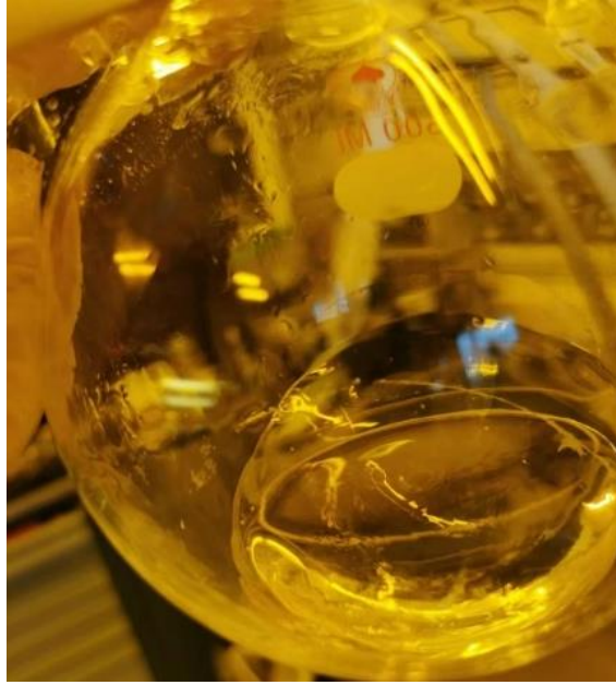
Figure 24. Purified transparent POMaC after overnight N 2 drying
