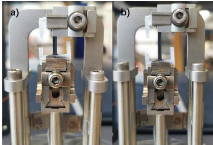
Figure 21. a) Unstretched POMaC/CIP sample fixed in DMA machine. b) Stretched POMaC/CIP sample at around 40% percent elongation.
