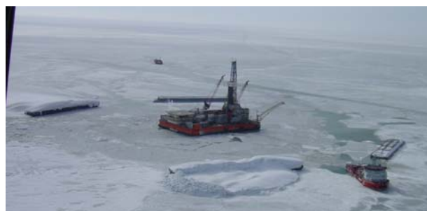
Figure 10 Exploration drilling barge protected by four IPS.
