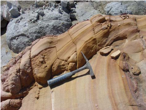
Figure 3 Weathering will cause the formation of new joints in massive rock that will affect the durability of the rock mass.
