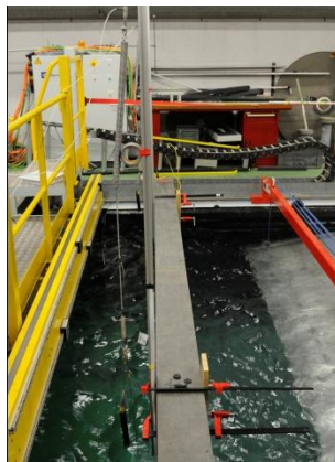
Figure A-2: Picture of the spring assembly to model the mooring lines stiffness
