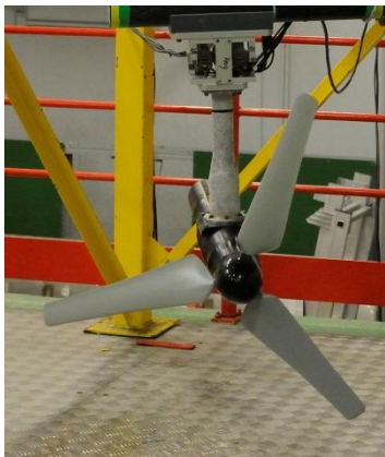
Figure A-1: Model of the turbine mounted on the vertical strut and load cell
