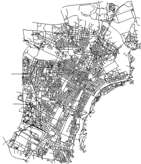
Fig. 2. The analyzed water distribution network.
