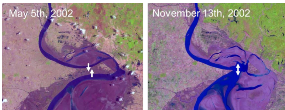
Figure B.9: Satellite images from May 2002 (left) and November 2002 (right) with the location of the meander cut-off indicated with arrows. As presented in (Arcadis, 2018). It indicates the volatile and dynamic behaviour starting downstream of the estuary entry point.
