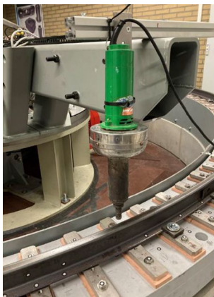
Fig. 2 The rails were cleaned and dried with a hot-air blower between the tests with FM-A and FM-B
