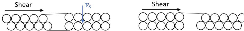
Figure 2.8: The dilatancy (left) and contractancy (right) by shear force on sediment bed, increasing and decreasing pore volumes
