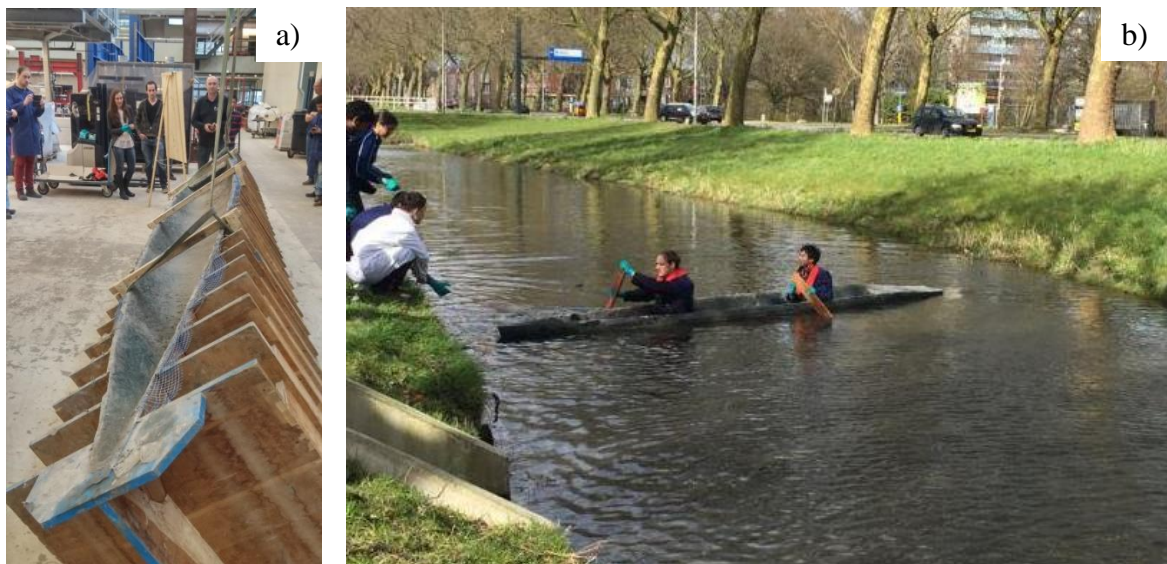
Fig. 15. a) Demoulding the canoe, b) watertightness test and trial ride of the canoe.
