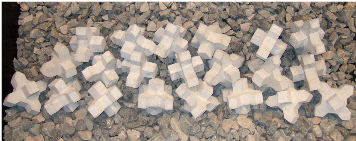
Fig. 5.30 second 0.3 D off centre placement
