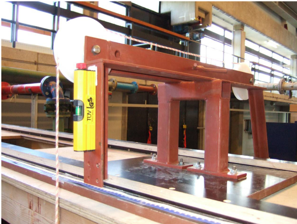
Fig. 5.3 moveable platform with “crane” mounted on top
