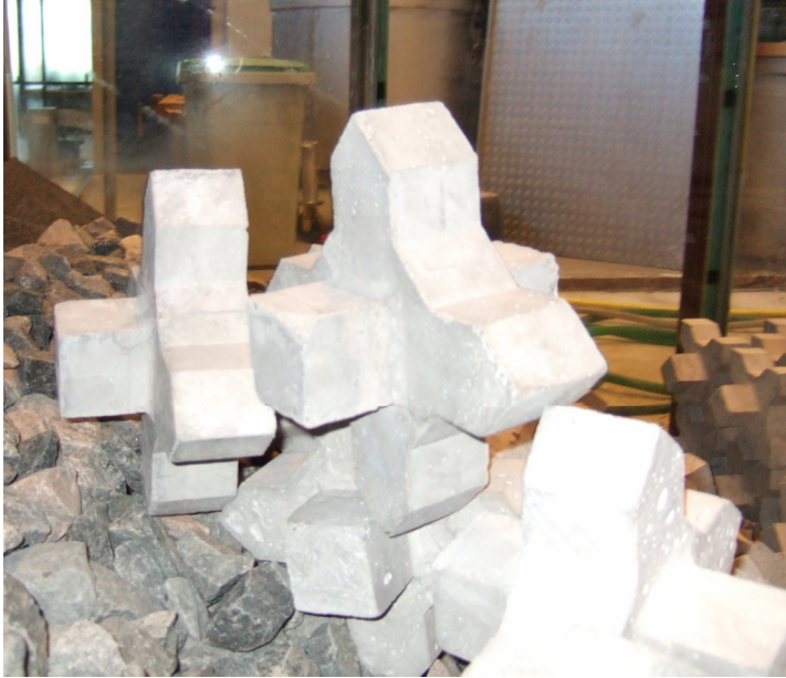
Fig. 3.5 unit placed partly onto other unit
