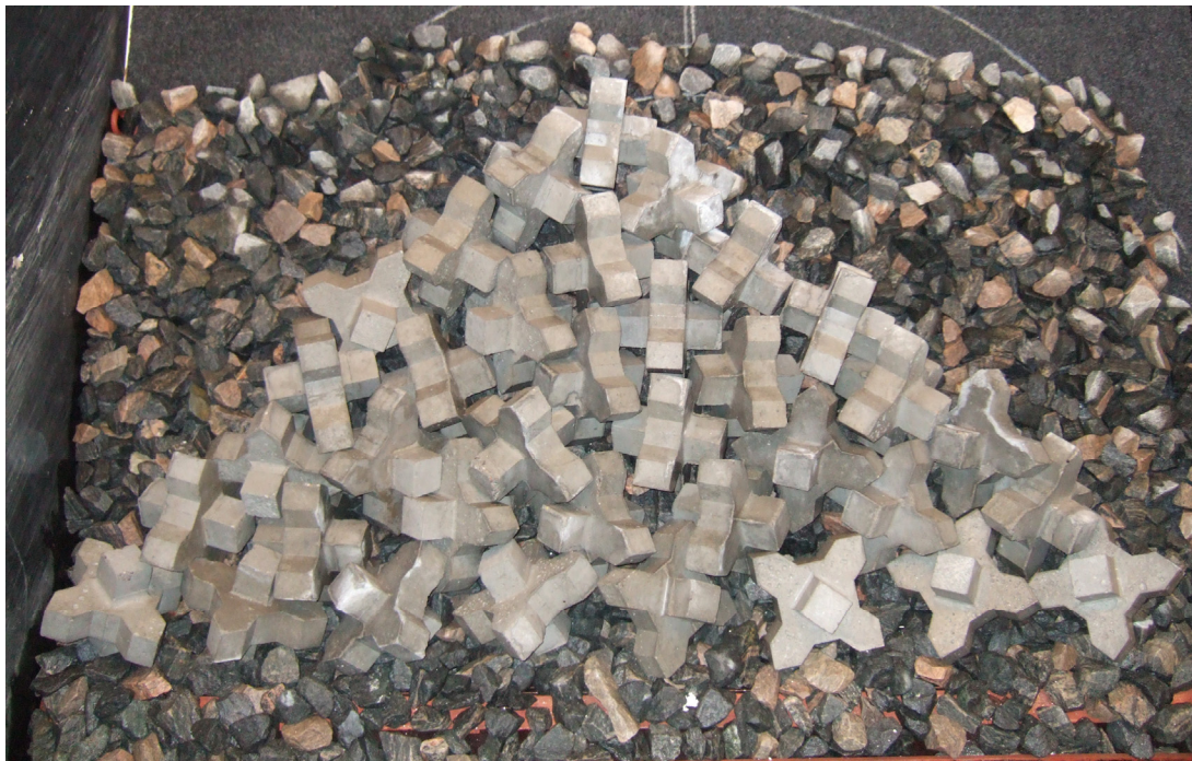
Fig. 5.21 picture of submerged placement test number two
