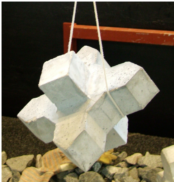
Fig. 4.1 Xbloc with three points pointing downwards
