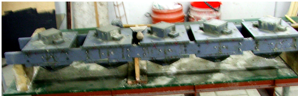
Fig. 5.5 reusable formworks of PVC
