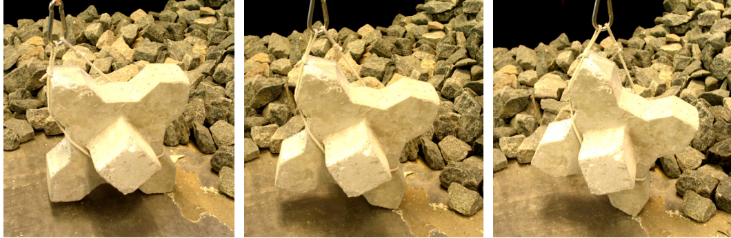
Fig. 4.4 rotation by lifting of the unit
