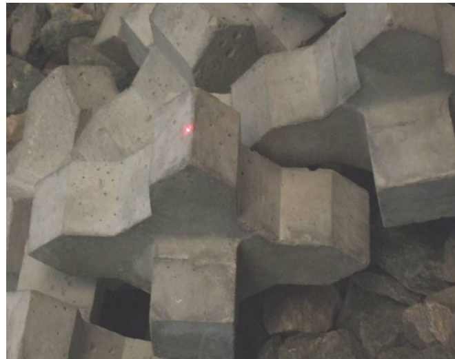
Fig. 5.4 laser dot pointing at centre of Xbloc unit
