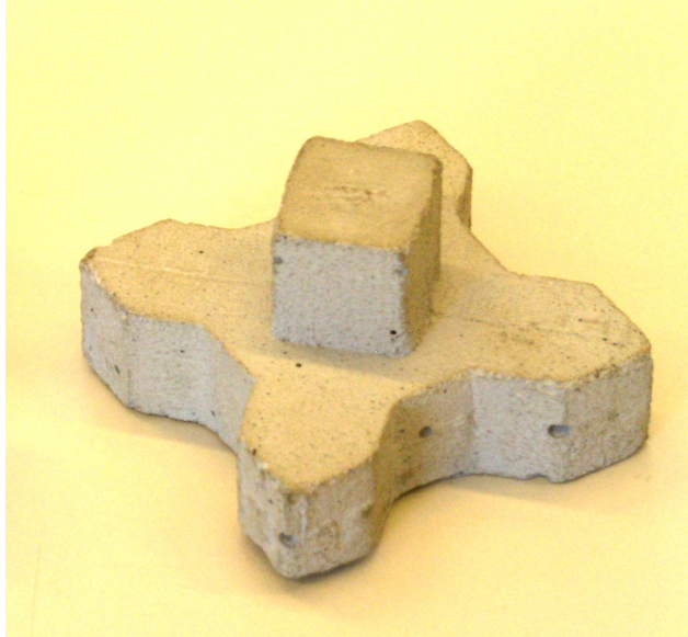
Fig. 6.15 special toe unit
