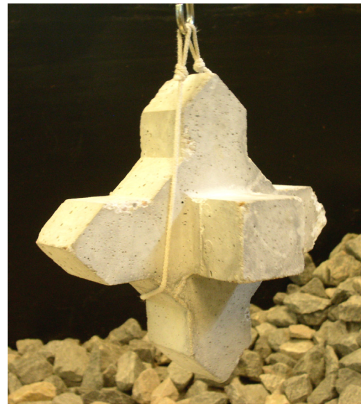
Fig. 4.2 Xbloc with one leg pointing downwards
