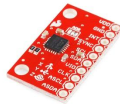
Figure 53. Image of the MPU-6050 mounted on the sparkfun breakout board
