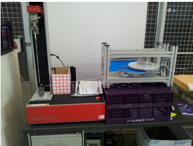
Figure 75. Showcase of the system used for measuring the forces of moving the bottom slide assembly. A pulley at the base of the tensile machine redirects the rope to the slide (Note: although in the picture the rope pulls the slide at an angle during the actual measurements this was not the case).
