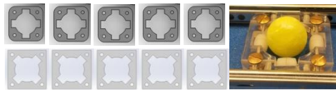
Figure 61 Showcase of the ball cages used to ensure that the ball cannot move away from its desired position.
