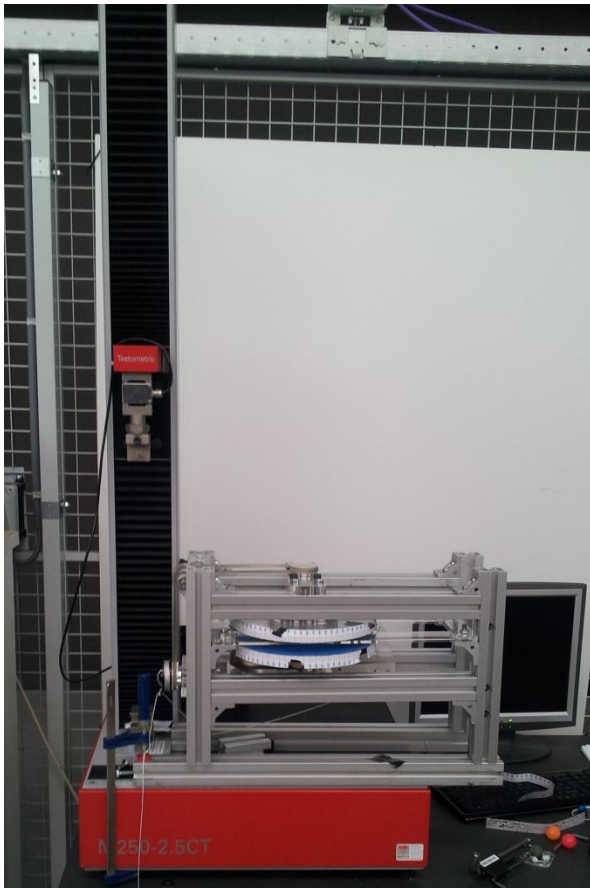
Figure 70. To generate hysteresis curves the Testometric M250-2.5CT tensile testing machine was used.
