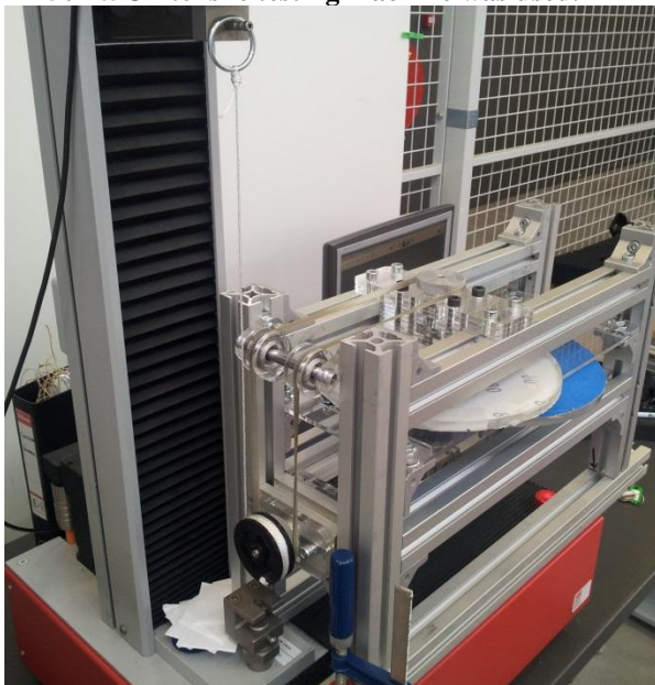
Figure 70. To generate hysteresis curves the Testometric M250-2.5CT tensile testing machine was used.
