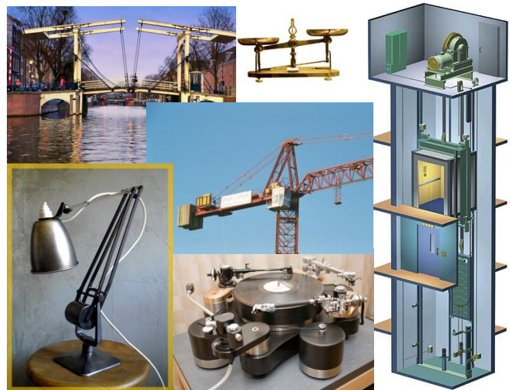
Figure 17: Various systems that are balanced against gravity by the usage of counterweights.
