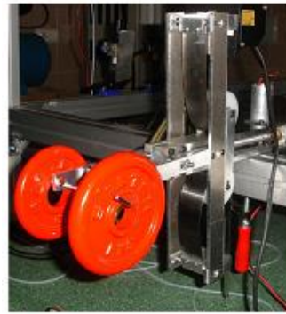
Figure 76: Assembled prototype of the AAC actuator. [24]
