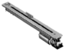
Figure 50. Image of the Alps motorized slide potentiometer
