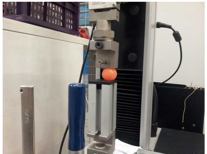
Figure 72. To measure the viscoelastic hysteresis curve of the ball that sits between the top and bottom disc, it was compressed and released a few times.
