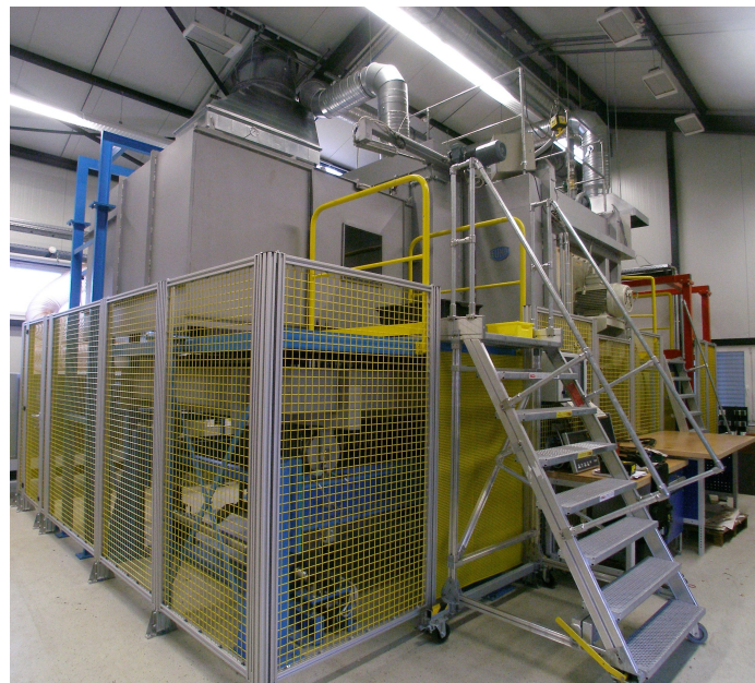
Figure 2.18: The glass bending furnace used by Fraunhofer IWM. [34].
