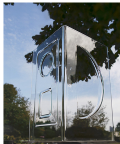
Figure 1.1: Glass deformed by laser bending [2].
