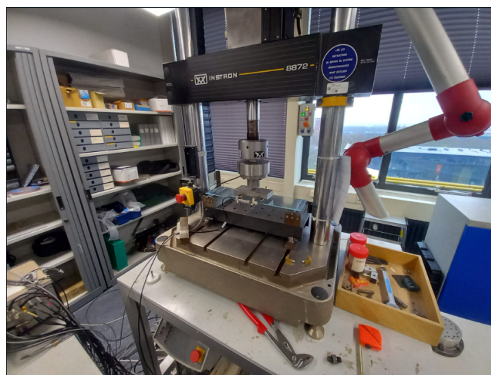
Figure 4.1: The Instron 8872 press used for the four-point-bending test.
