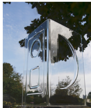
(b) Glass deformed by laser-forming [2].
