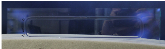
(a) Captured residual stress in bend corners.
