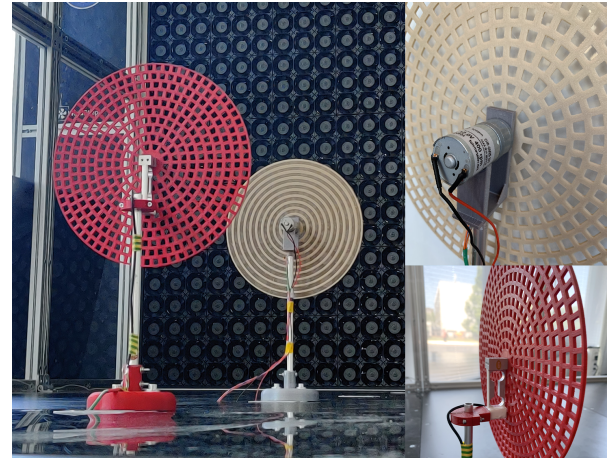
Figure 5: The test set-up as used in the Windshaper with the Helix porous disc (white) mounted at 5D upstream of the sensor porous disc (red). The top right image shows the DC motor used in the experiment. The bottom right image shows the load-cell and its mounting hardware.
