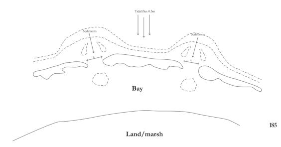
Schematic representation of barrier islands, parallel to the coast line, longitued island formation, and same inlet spacing.
