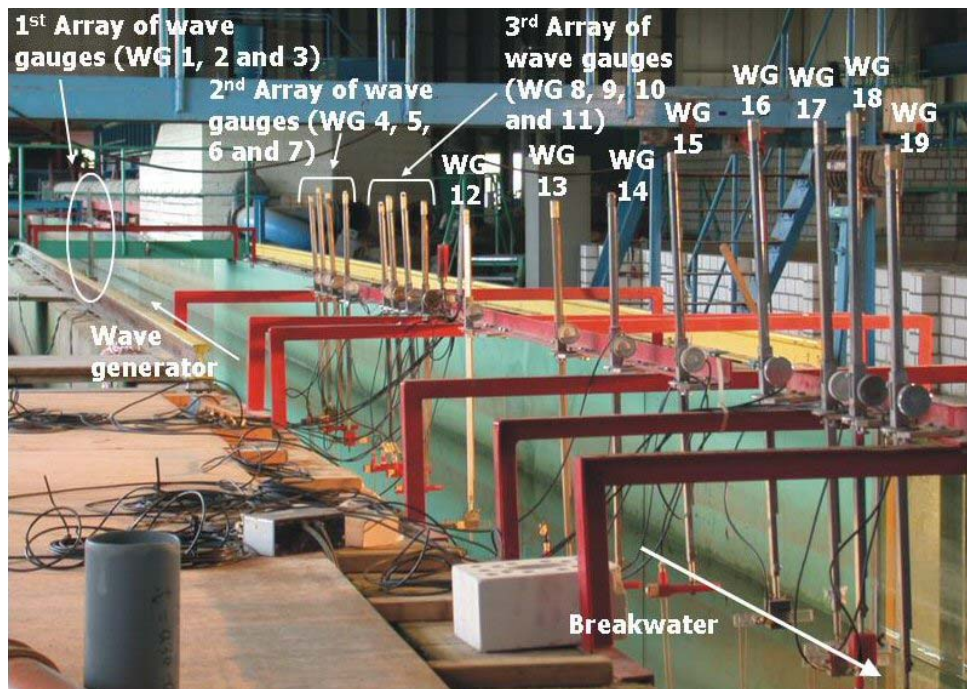
Figure 11: Wave gauges in the wave flume for determination of wave parameters
