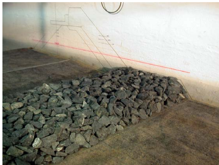
Figure 17: Photos of the construction of the model at LWI: foreshore construction (left) and breakwater toe (right)
