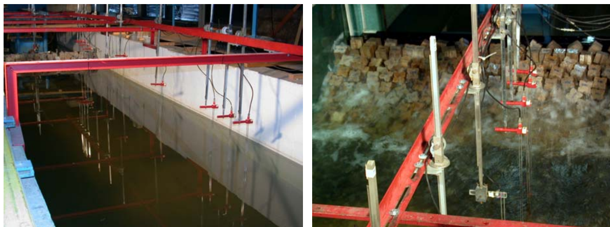
Figure 19: Wave gauges in front of the model at LWI: before (left) and during tests (right)
