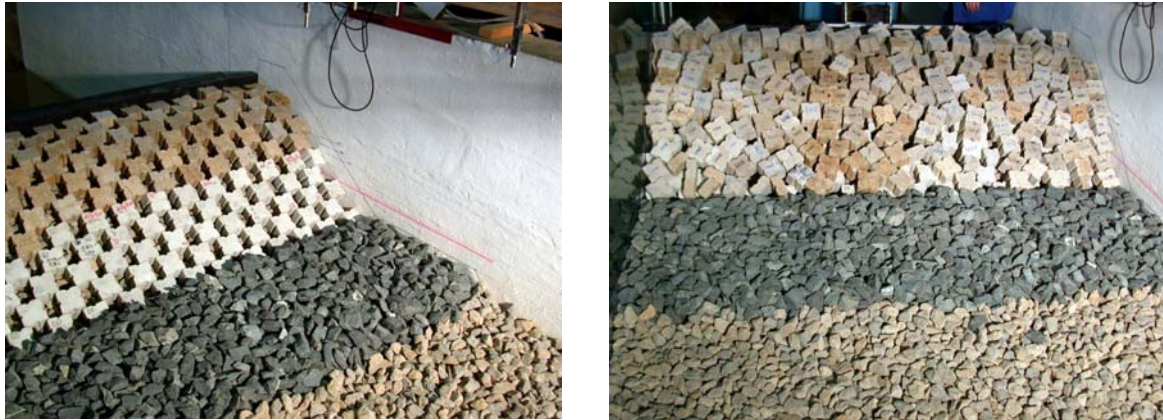
Figure 18: Construction of the top layer of the model at LWI: first layer (left) and top layer (right)
