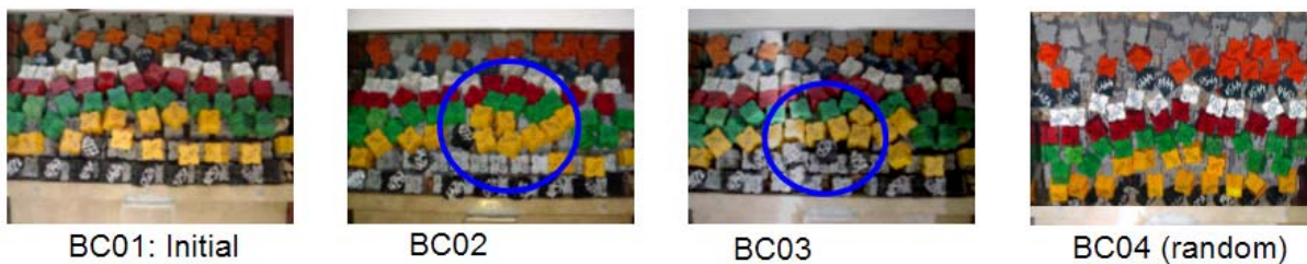
Figure 44: Spatial variability changes in the upper armour layer after the foreshore change
