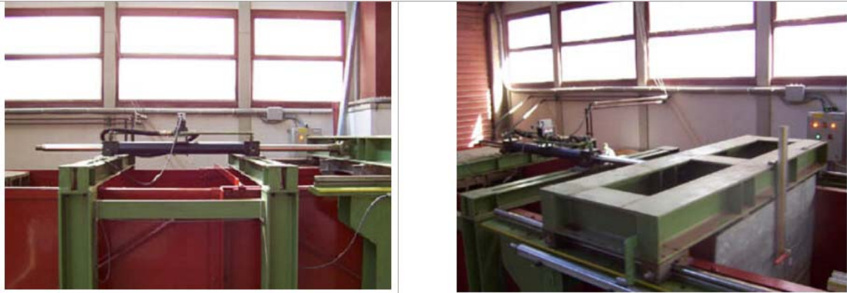
Figure 24: Wave generation system of the UPVLC wind and wave test facilities
