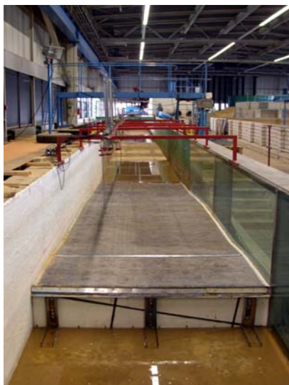
Figure 17: Photos of the construction of the model at LWI: foreshore construction (left) and breakwater toe (right)
