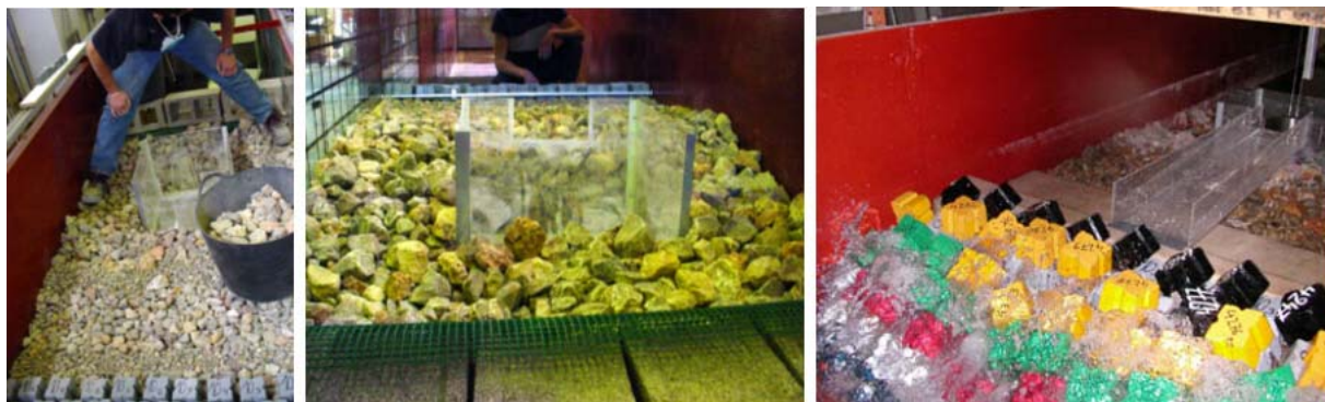
Figure 36: Overtopping measurement setup at the UPVLC
