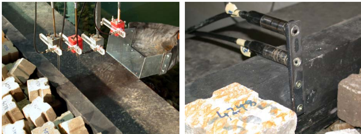
Figure 21: Velocity measurements of individual overtopping volumes by means of layer thickness gauges (left) and pressure measurements on a dummy “person” (right) at LWI model
