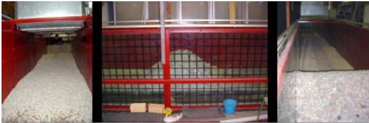
Figure 28: CLASH foreshore in the UPVLC Zeebrugge scale model
