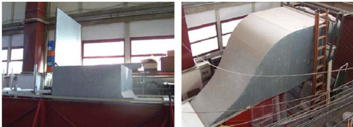
Figure 25b: Air intake and blowers of the Wind Generation System (UPVLC)
