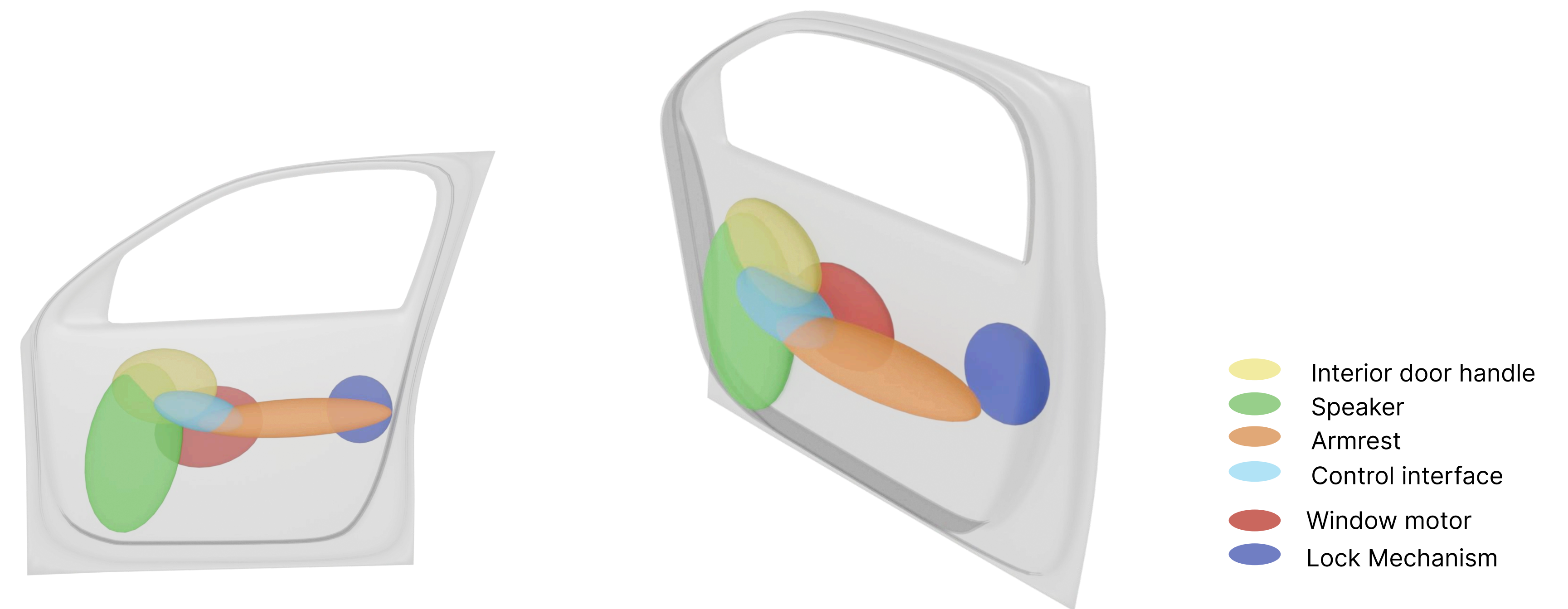
Figure 31 - Visual model of location of components
