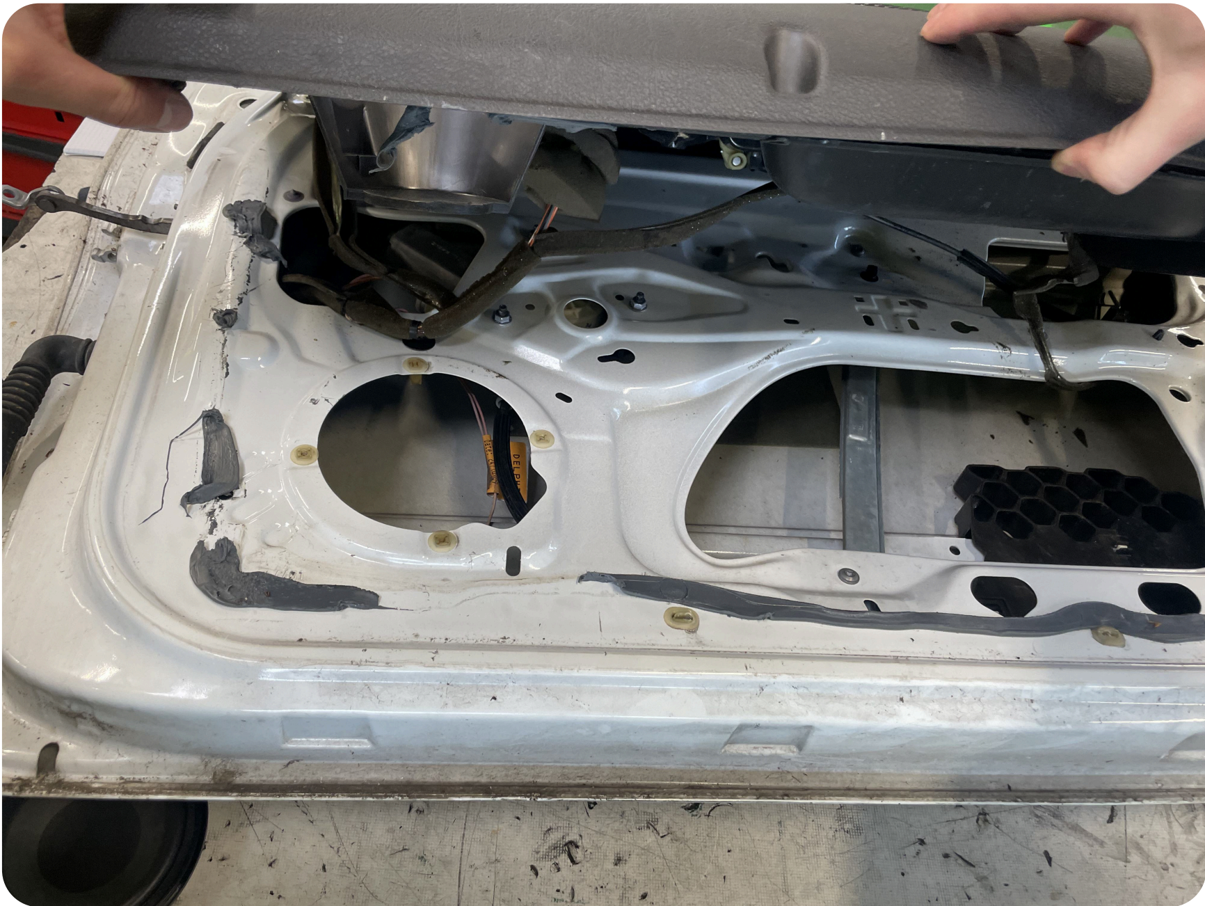
Figure 24 - Process of removing the interior panel Door A
