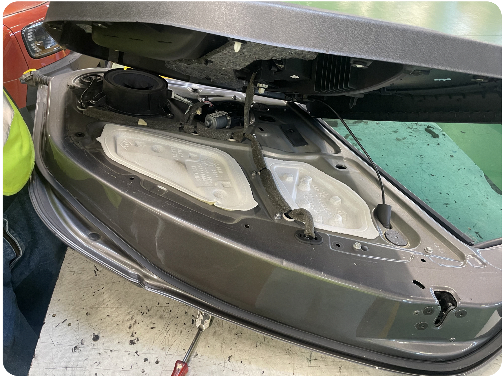
Figure 25 - Process of removing the interior panel Door B
