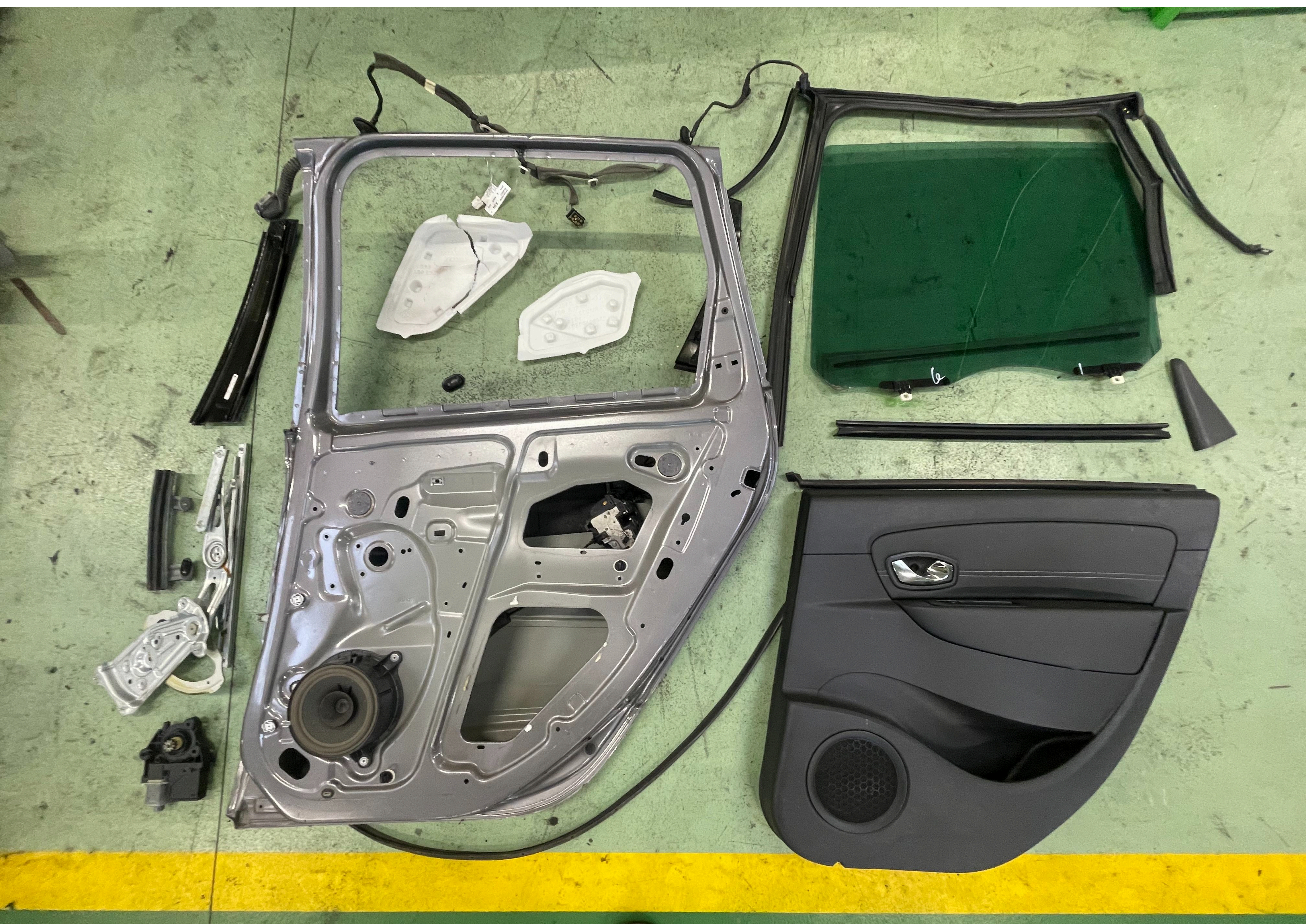
Figure 22 - Door B disassembled and legend of disassembly map
