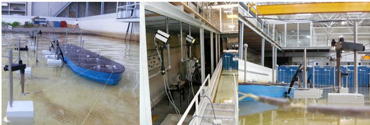
*Figure 3. Oil tanker model moored to the berthing structure (left); Qualisys motion capture system (centre); force transducers for mooring line and fenders' forces measurements (right).*
