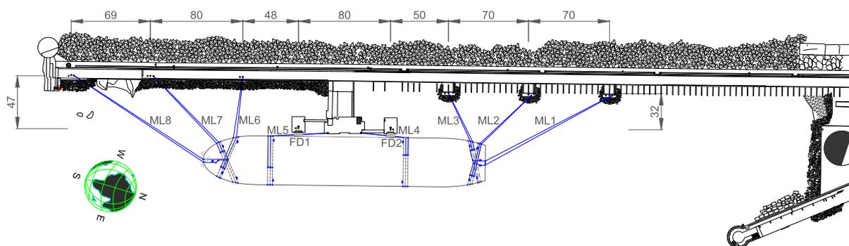
Figure 8. Symmetrical mooring layout used in the physical model tests.
