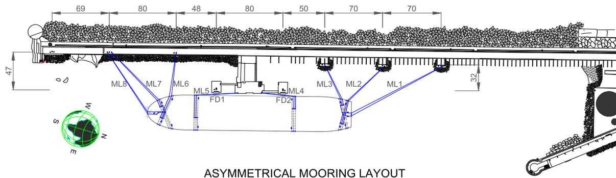
Figure 2. Usual ship mooring layout at the Berth “A” Oil Terminal.
