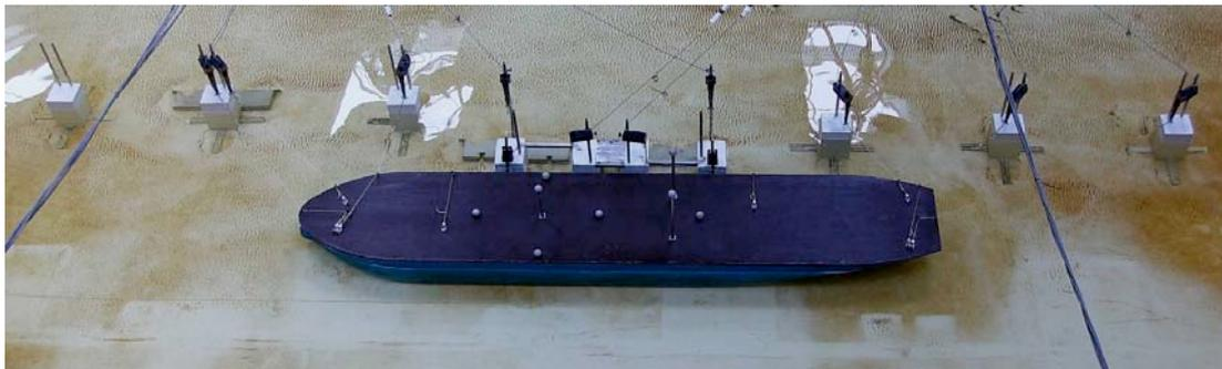
*Figure 4. Ship model moored to the berthing structure (asymmetric mooring layout): first phase of the study.*
