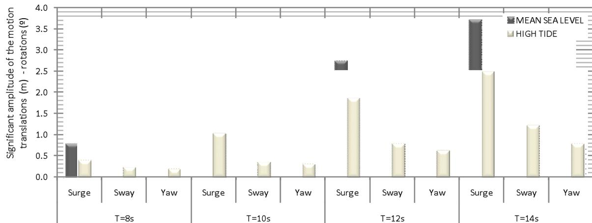
Figure 10. Significant amplitude of the horizontal moored ship motions for the two water levels studied: mean sea level and high tide water level.
