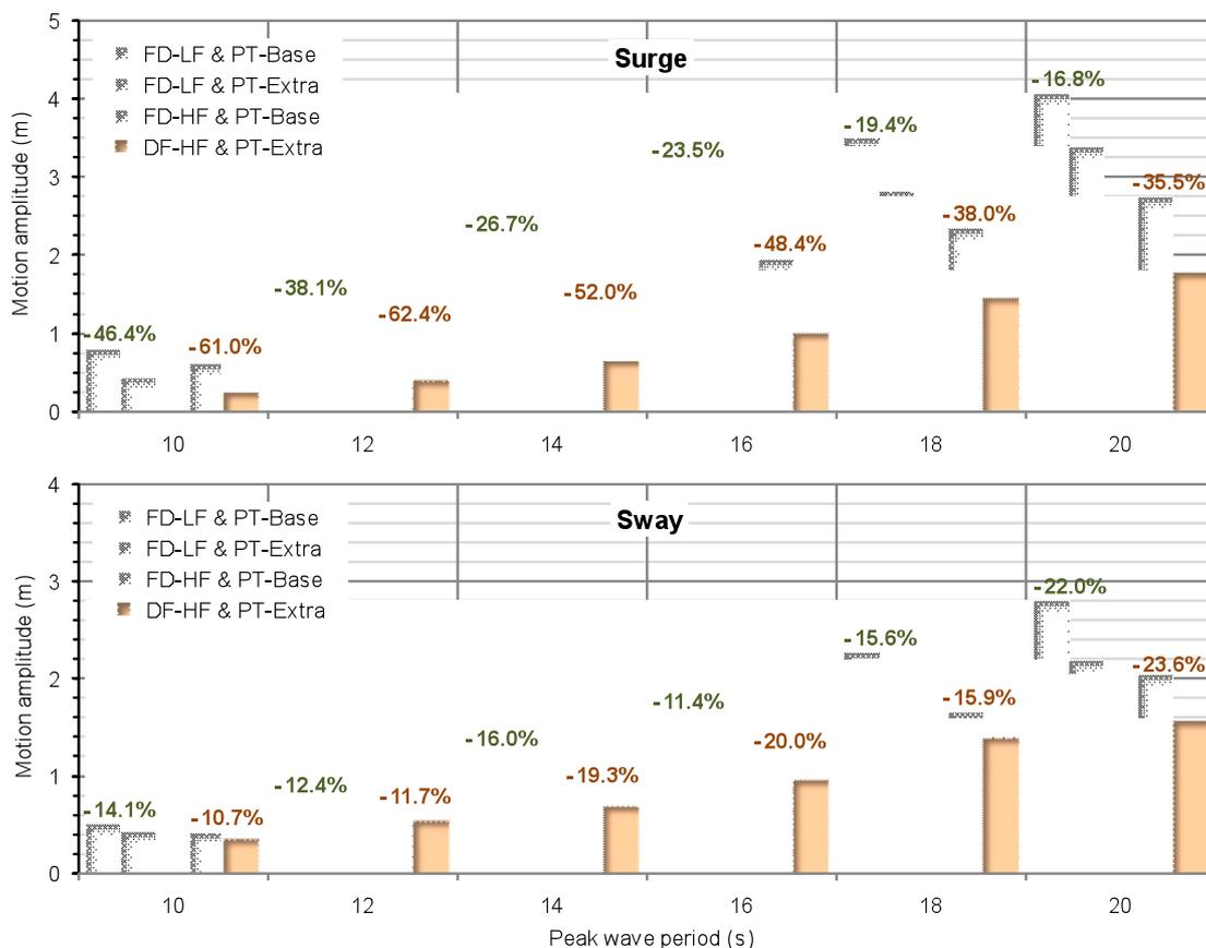
Figure 12. Significant amplitudes of surge (upper) and sway (down) motions for different characteristics of the mooring system. Results of the second phase of the study.
