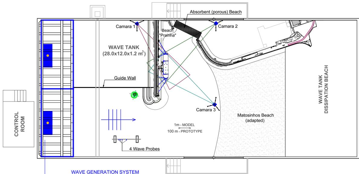
Figure 6. Physical model set-up in the wave tank: second phase of the study.
