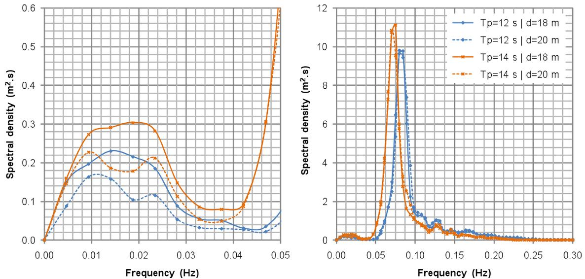
Figure 11. Influence of the water depth,  $d$ , in the infra-gravity energy content of two sea state conditions measured in the wave tank: low frequency band (left), complete spectrum (right).
