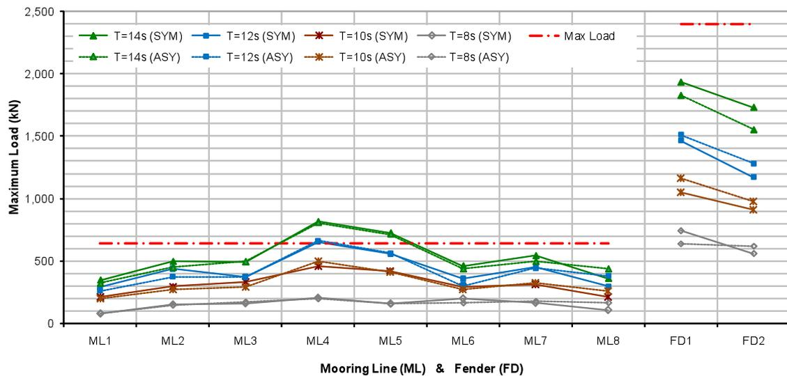
Figure 9. Maximum loads on the ship mooring lines and fenders for the asymmetrical and symmetrical mooring layouts.
