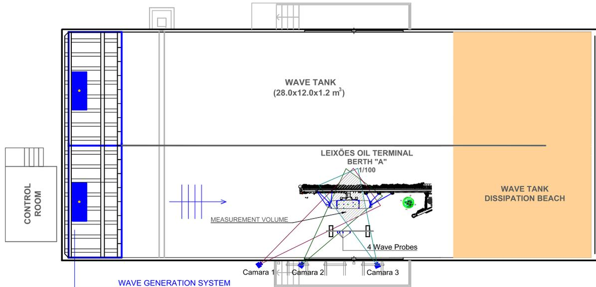
Figure 5. Physical model set-up in the wave tank: first phase of the study.
