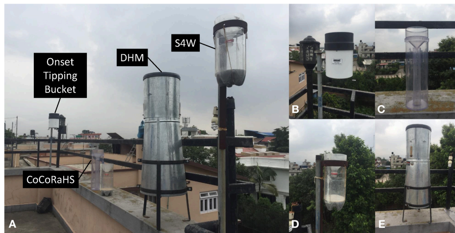
FIGURE 4 | Comparison between (A) four different gauges including: (B) Onset Computer Corporation Hobo tipping bucket, (C) Community Collaborative Rain, Hail, and Snow Network (CoCoRaHS) standard 102 mm (4-inch) diameter gauge, (D) S4W gauge, and (E) the Nepali Department of Hydrology and Meteorology (DHM) standard 203 mm (8-inch) diameter gauge (similar to a US National Weather Service 203 mm (8-inch) gauge).
