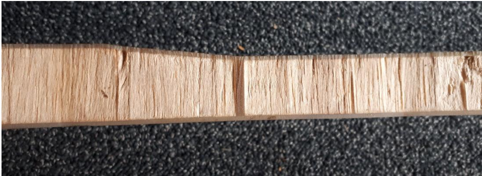
Picture 21, Thickness change of core material.
