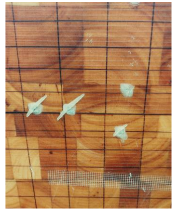
Picture 34. Impact test. Most right picture shows the damage created by the air rifle.
