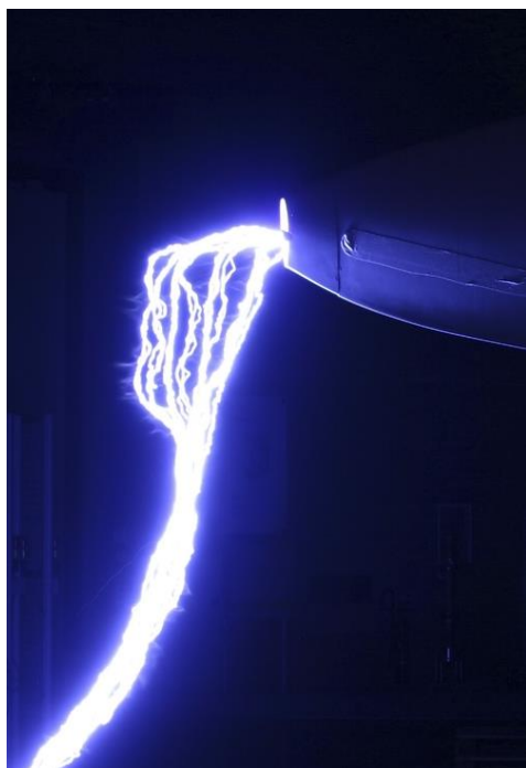
Picture 30. Wind turbine blade being tested on lighting strikes. Photo credit: LM Wind Power.
