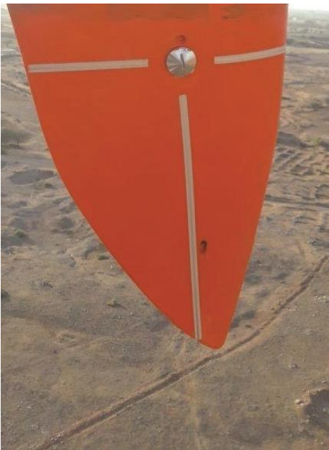
Picture 27. Exterior lighting diverters on a wind turbine blade (Hall, 2021). Image credit: Weather Guard Lightning Tech.
