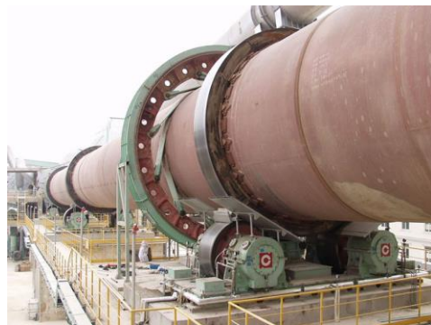
Picture 5 Rotary kiln which is used for cement production. Picture from heavy-plant..com (n.d.) The kiln is only one step of the entire cement production process.
