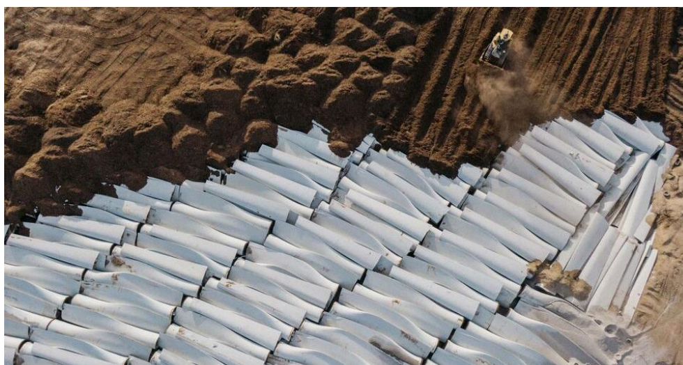
Picture 3. Wind turbine blades being covered by dirt in a landfill. Benjamin Rasmussen (2020) for Bloomberg Green
