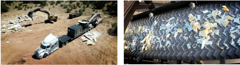
Picture 10. Portable wind turbine blade recycling solution (left) and shredded wind turbine blade (right). Image credit: ssiworld.com (2023).
