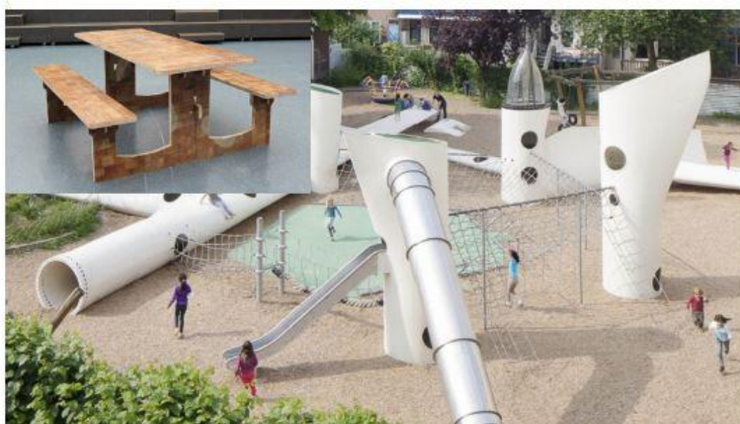
image / figure 1 Table and playground made from old wind turbine blades.
