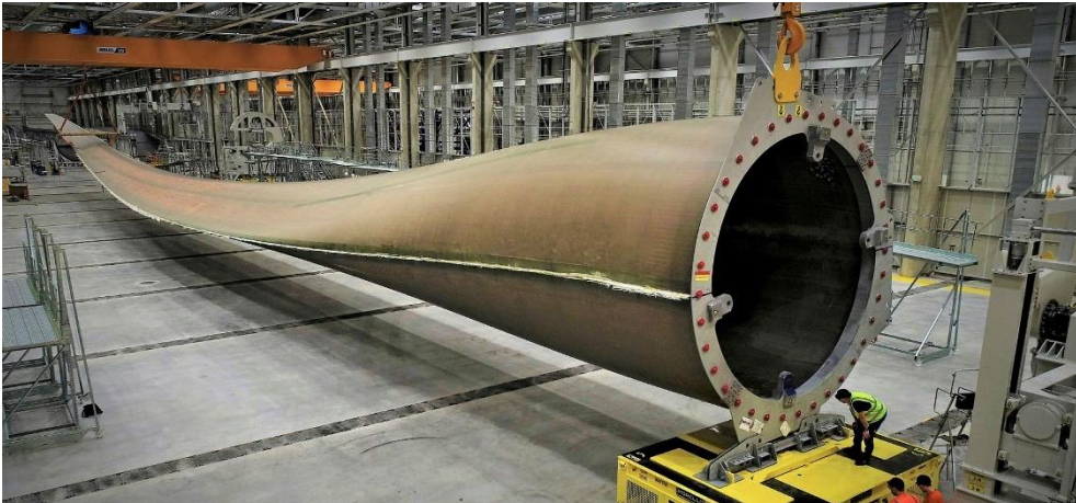
Picture 24. The GE/LM Wind Power LM 107.OP wind turbine blade with the three aspects visible (ge.com, 2019). Image credit: GE Renewable Energy
