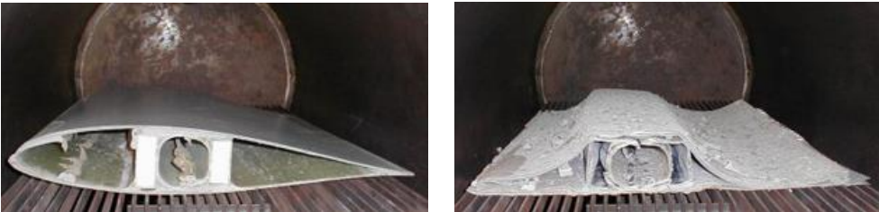
Picture 11. Thermal decomposed wind turbine blade (pyrolysis), left: before, right: after. Image credit: refiber.com (n.d.).
