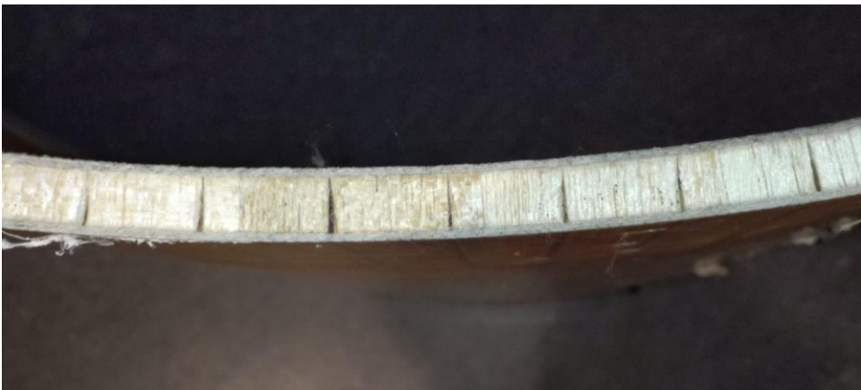
Picture 22. Side view of core with kerfs.
