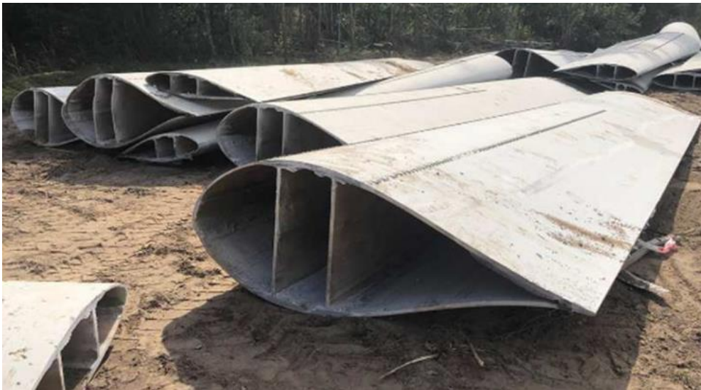
Picture 20. Cross section of a wind turbine blade with a shearweb design (Juntikka et al, 2018)
