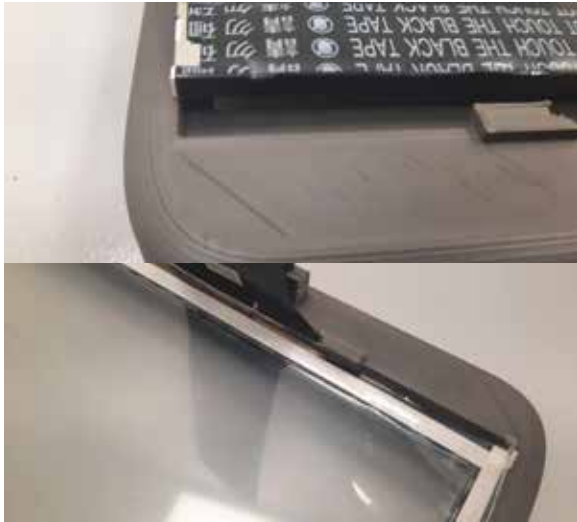
Figure 63: Too small 'inside housing'
