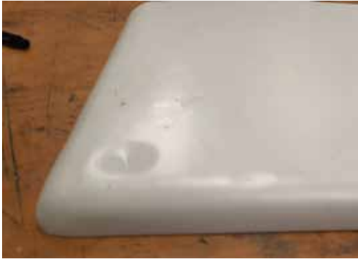
Figure 55: Unclear cutout for the 'feet'
