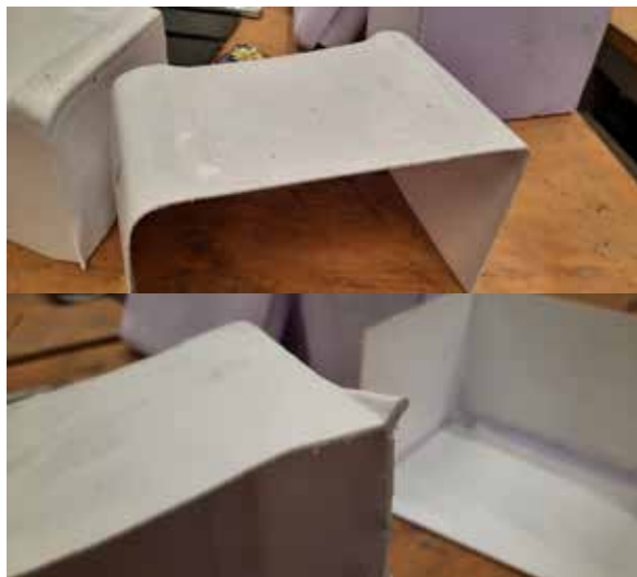
Figure 52: Top: unclear cutout Bottom: excess material
