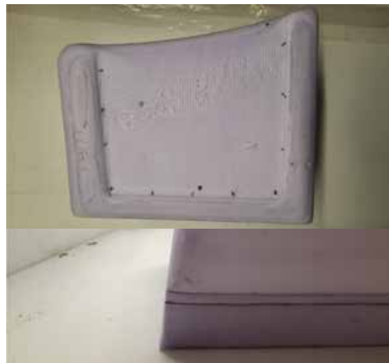
Figure 53: Top: holes in the thermoform mold Bottom: Tapered mold
