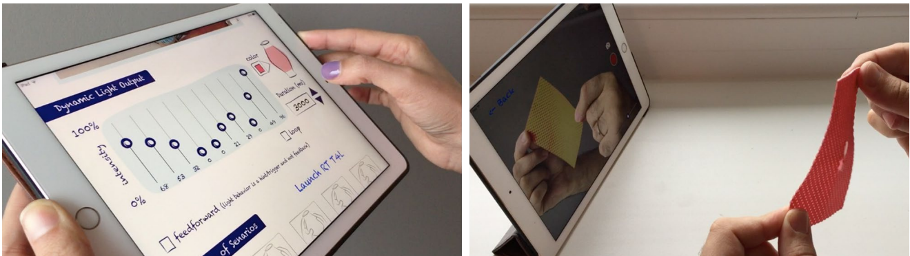
Figure 13. The real-time Chroma-key app: a snapshot of the interface (left), the user can select the color by touching it on the screen and use the slider to fine-tune the threshold (right).
