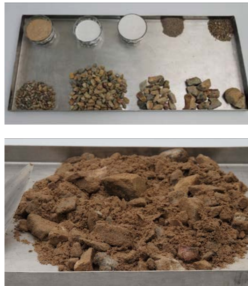
Figure 2.2. Aspect of soil GN: soil fractions (up), and soil mixed with water (down) (Correia dos Santos, 2014).
