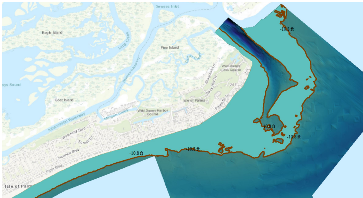
Figure 7.4: The contour line for the depth of closure (10.8 ft). March 2009.
