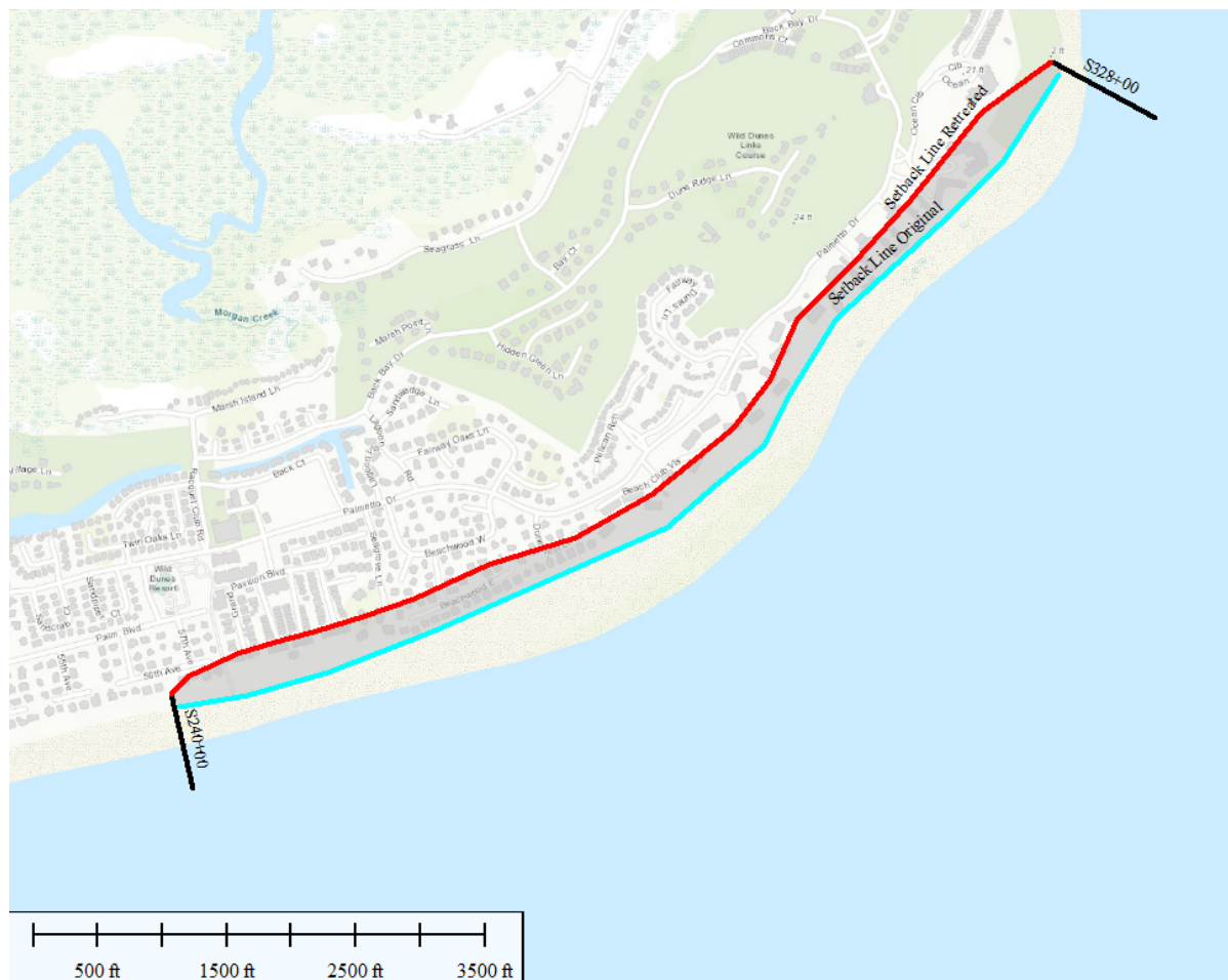
Figure 10.5: Example of redrawing the setback lines. The light blue line is the original setback line, the red line is the new proposed setback line.
