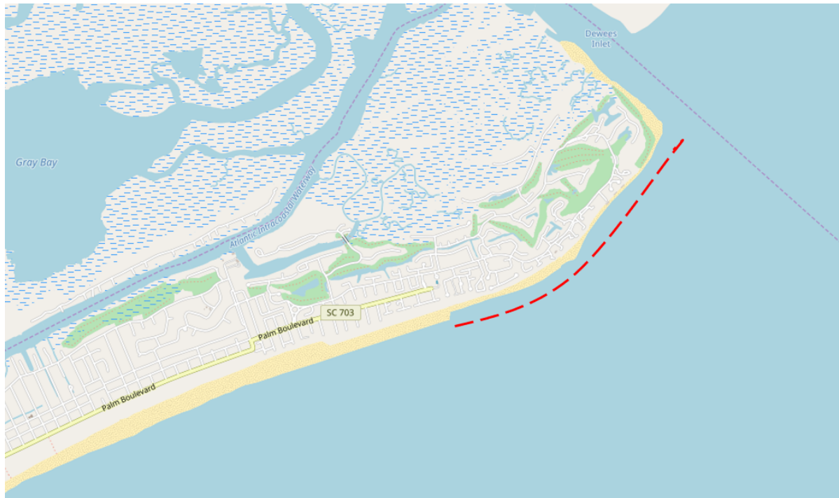
Figure 10.11: Design for the offshore breakwater placement. The offshore breakwaters in red along the coastline
