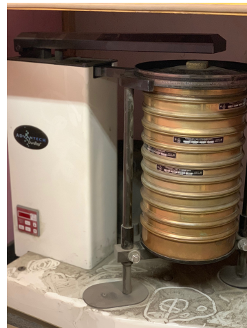
(b) The sieves on a vibrating mound.
