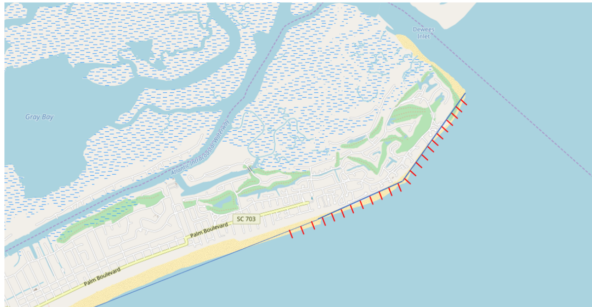
Figure 10.10: Design for the groynes. The groynes in red, in the part of the beach with the most erosion problems
