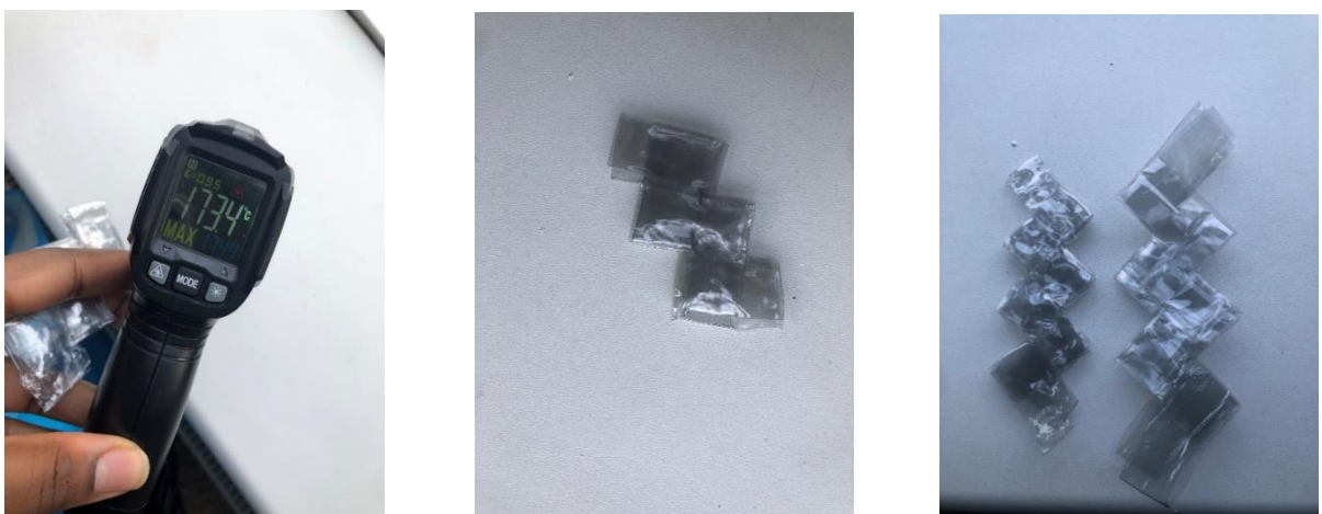
Figure 89: Heat application and infrared thermometer measurement
