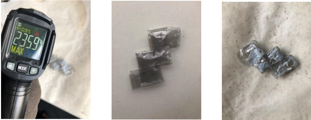
Figure 90: Heat testing above glass transition temperature and measurement with infrared thermometer
