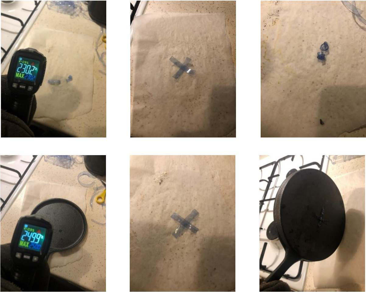
Figure 85: Testing the prototypes and measuring the temperature of the metal press
