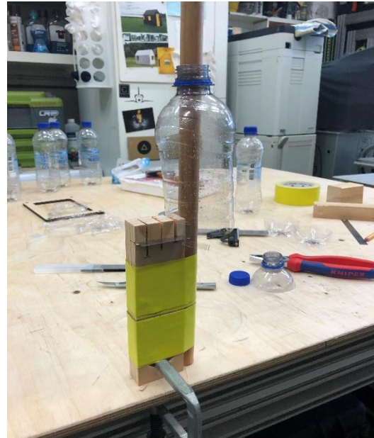
Figure 73: PET slicer with a pole attached for ease of slicing
