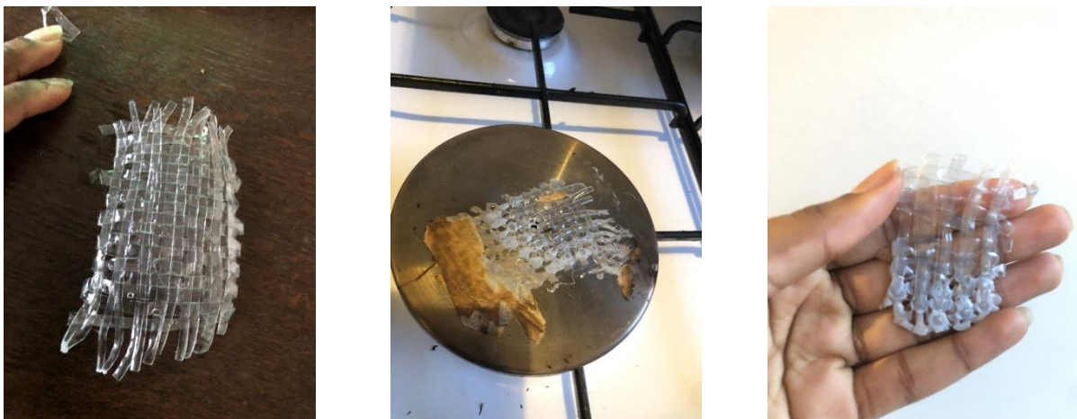
Figure 81: Heat test with baking paper, iron and metal base
