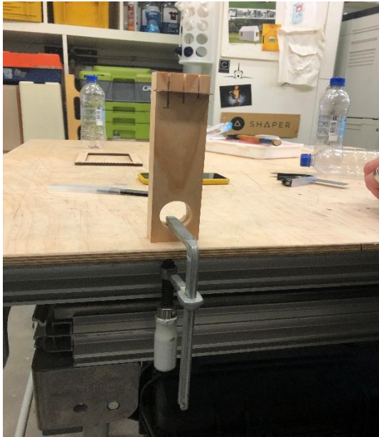
Figure 74: First PET slicer model with 20, 25 and 30mm space for thread
