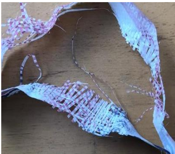
Figure 99: Cement bag and woven plastic after the tensile strength testing
