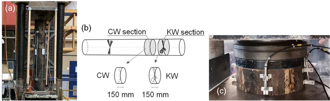
**Figure 1.** Test set-up: (a) compression test of large-scale pile segments, (b) extraction of 150 mm thick discs from a clear wood (CW) section and a section with knots (KW), and (c) small-scale compression test of a disc with knots.
