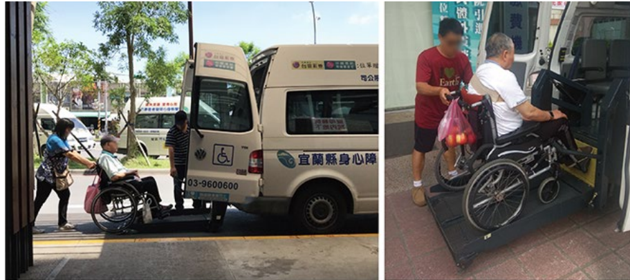
Figure 1 A driver of the long-term care shuttle vehicle helping an elderly citizen on board with the wheelchair lift (photo provided by the authors).
