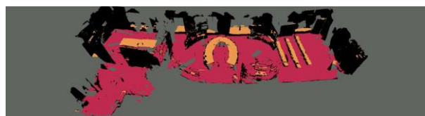
Figure 3: Object oriented visualization. Orange: obstructive objects. Black: walls. Red: floors
