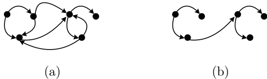
Figure 2: A quasi-strongly connected graph (a) and one of its directed spanning trees (b)
