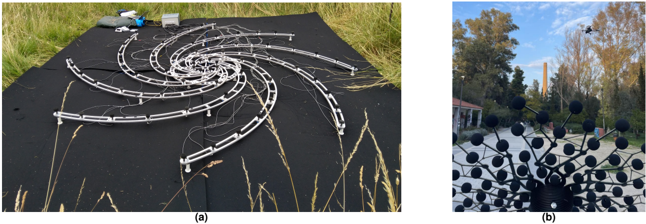
Figure 2: Examples of the microphone arrays employed in field measurements. (a) 64-microphone array (PUI Audio 665-POM-2735P-R) distributed in a multi-arm spiral configuration. (b) CAE Bionic M-112 microphone array measuring the noise emissions of a hovering drone.
