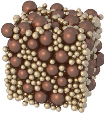
Figure 5.5 HADES simulation of a 3-dimensional container filled with 30% [ \text{m}^3/\text{m}^3 ] 4 mm spheres and 70% [ \text{m}^3/\text{m}^3 ] 10 mm particles.
