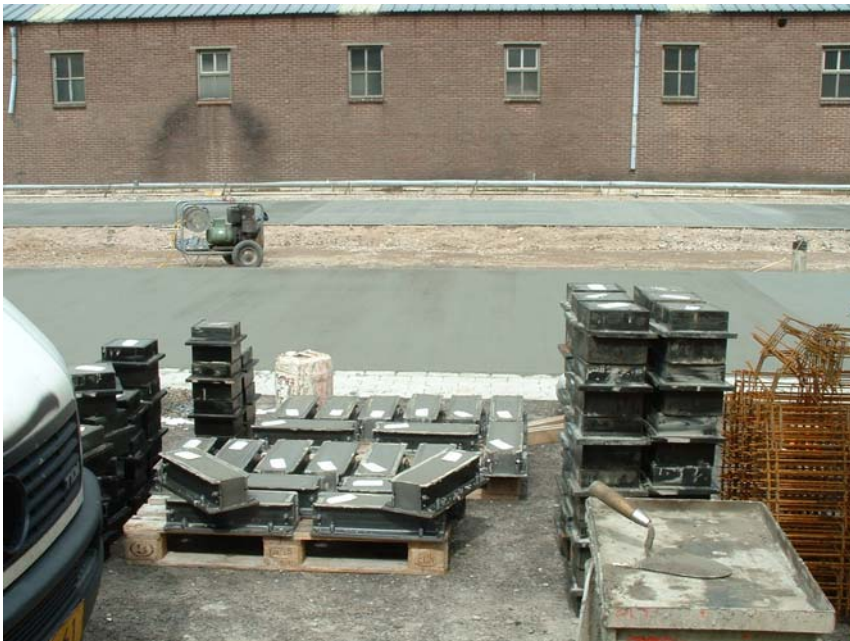
Figure 8.18 Additional specimens for laboratory testing were cast simultaneously with the same mixtures.
