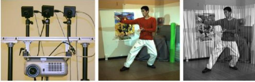
Figure 11: The 3D video brick with cameras and projector (left), simultaneously acquiring textures (middle) and structured light patterns (right)
