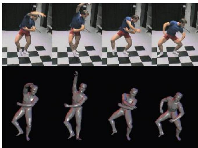
Figure 5: From eight video cameras spaced all around the scene, model-based method can capture the complex motion of a dancer.
