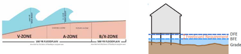
FIGURE 5.6 Left: FIRM flood zones based on inundation level and wave exposure (NYCDP, 2013a). Right: The Design Flood Elevation (DFE) is the minimum elevation, based on the sum of the Base Flood Elevation (BFE) and a freeboard based on the building's structural category (NYCDP, 2014b)
