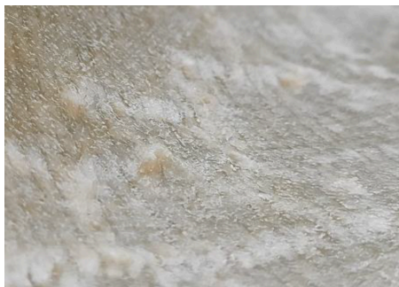
Figure 9: Fibre buckling on experiment 1
