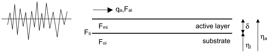
Figure 3.1: The active layer model of Hirano (1971), after his Figure 2, p.194.
