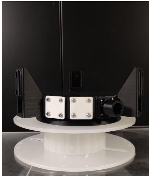
Figure 30. The 3D printed respiratory bellow connector with the 3 mounted frame connectors. The tube socket that are not in used are sealed with the seal connectors, 3D printed with white TPU 95A.
