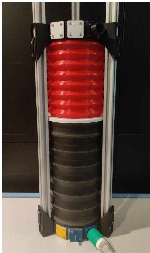
Figure 31. The physical respiratory-abdominal model developed in the context of this thesis.
