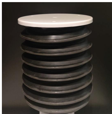
Figure 25. The latex bellow used as the abdominal component in the model.
