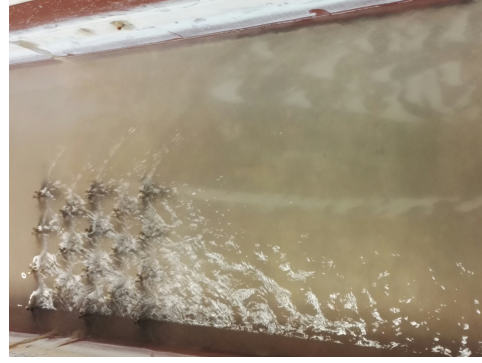
Figure 4.11: Retardation behind partly blocked flow
