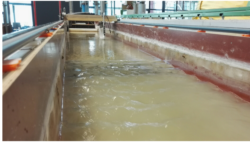
Figure 4.20: Impoundment of water level by porcupines, Experiment 8
