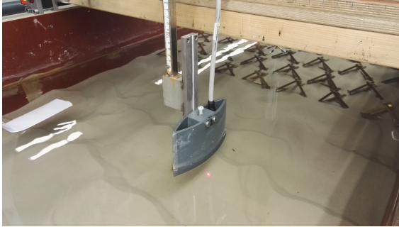
Figure 3.9: Laser measurement in a special boat such that it can measure under water
