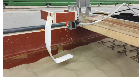
Figure 3.10: Laser measurement that determines the water level by using a piece of paper
