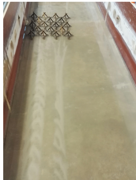
Figure 4.4: Two strokes of sedimentation behind staggered porcupines
