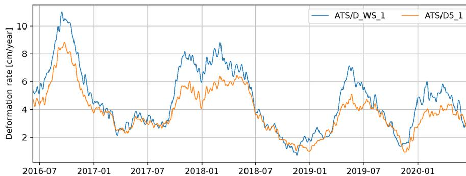
**Figure 2.** Daily deformation rate of the Vögelsberg landslide at benchmarks “D5\_1” and “D\_WS\_1” (Fig. 1), as measured by the automated total station and smoothed by a moving average filter over the last 32 d.
