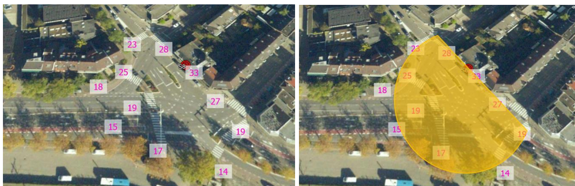
Figure 11: Average RSSI values around sensor8 (left) and its range shape (right)
