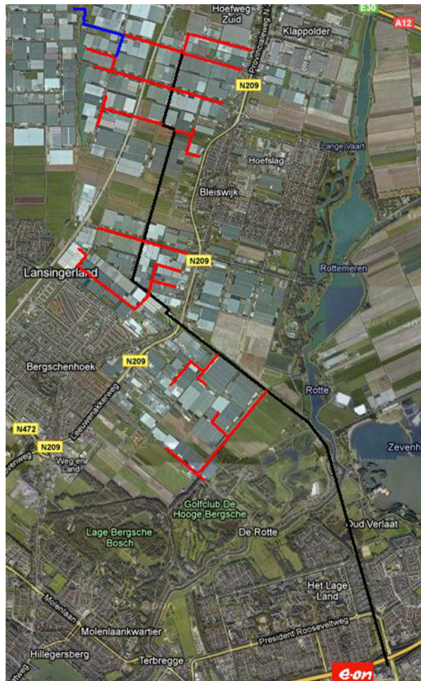
Figure 1.1: The old situation with the pipeline of RoCa in black and the pipelines to the greenhouses in red. (Arcadis, 2012).
