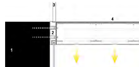
Fig. 217. Catwalk and earth volume connection. (1) Unstabilized poured earth; (2) Internal door frame system; (3) Hotel room entrance doors; (4) Catwalk
