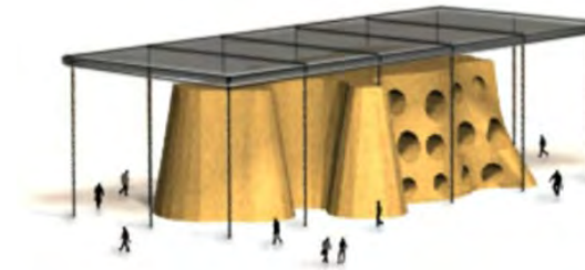
Fig. 148. Earth volume covered with glass roof on steel columns
