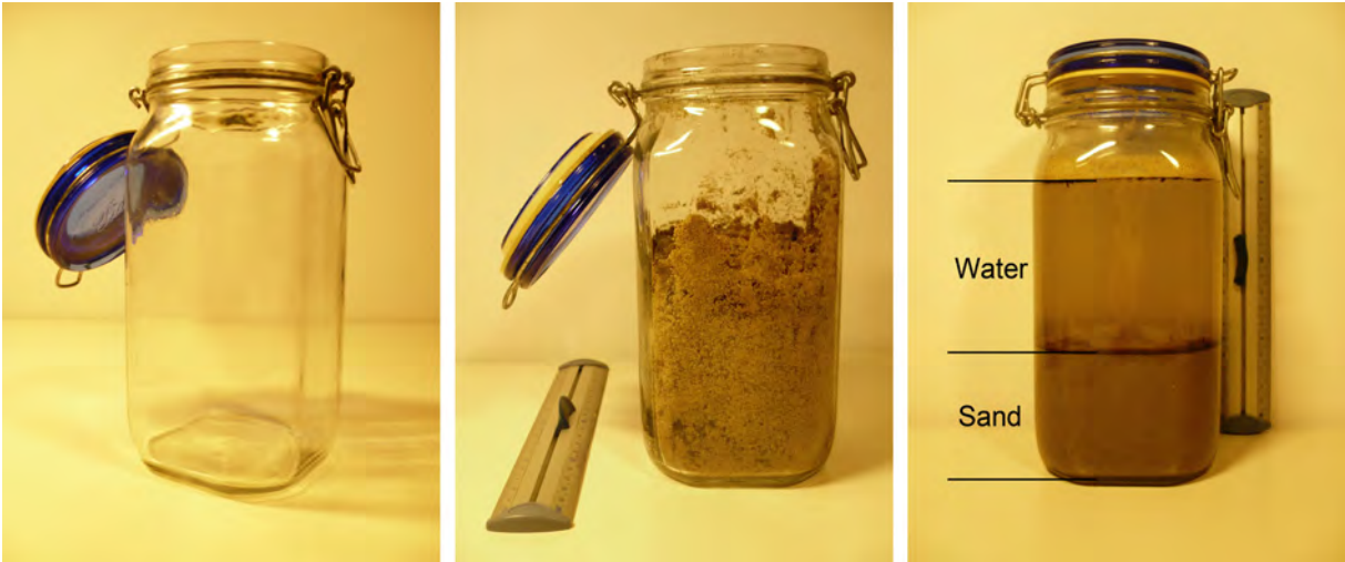
Fig. 28. Sedimentation test with soil sample Nr. 2
