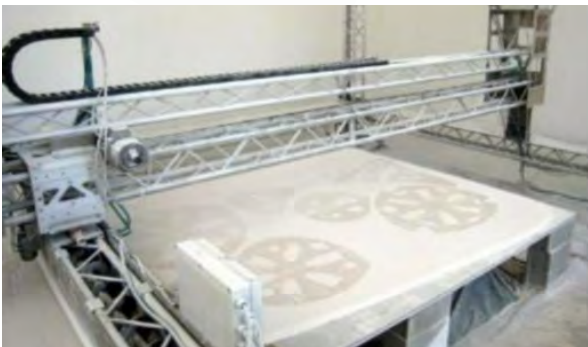
Fig. 118. 3D earth printer in action
