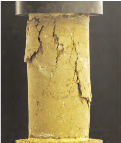
Fig. 50. Compression test results of circular specimens
