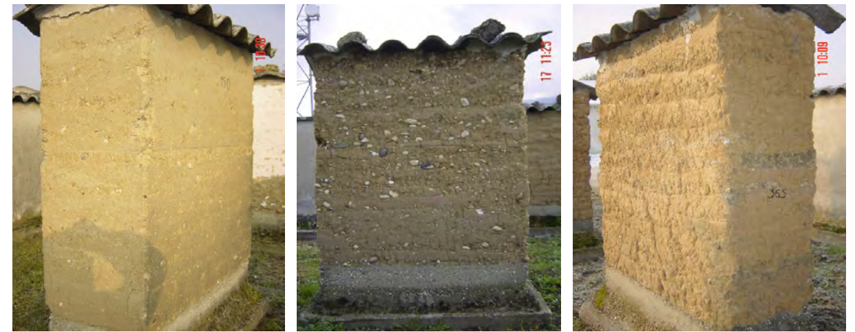
Fig. 63., 64., 65. Rammed earth specimens after aging for 20 years. Left – stabilised (5% lime), middle and right – unstabilised
