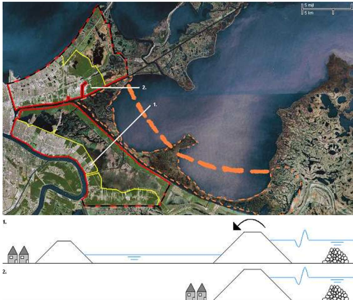
Fig. 3.17: Breakwater alternative
