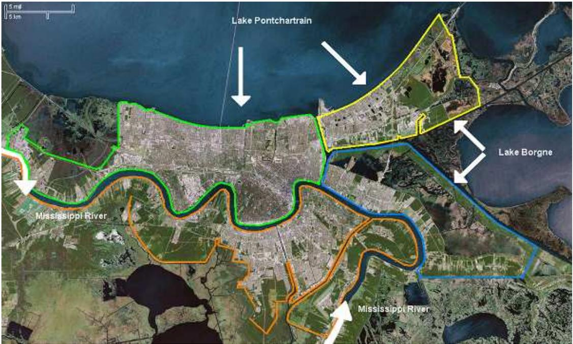
Fig. 2.8: The dike ring areas of New Orleans, in combination with their direct water threat
