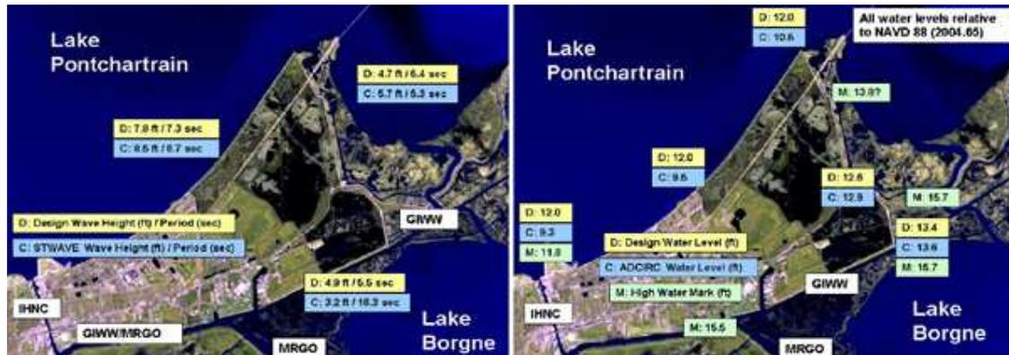
Fig. A.11: Left – Eastern section of Orleans Parish: comparison of wave maxima with design values [31]
