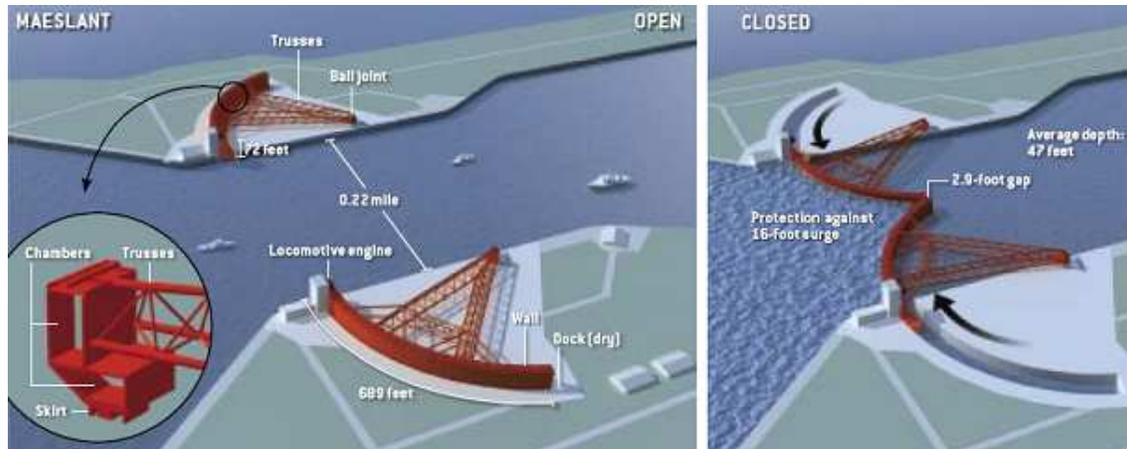
Fig. D.7: New Waterway Storm Surge Barrier – Design with floating sector gates [14]
