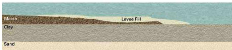
Fig. C.11: Overtopped levee erosion failure mechanism [1]
