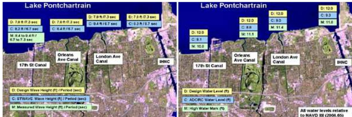
Fig. A.10: Left – Jefferson and Orleans Parishes: comparison of wave maxima with design values [31]
