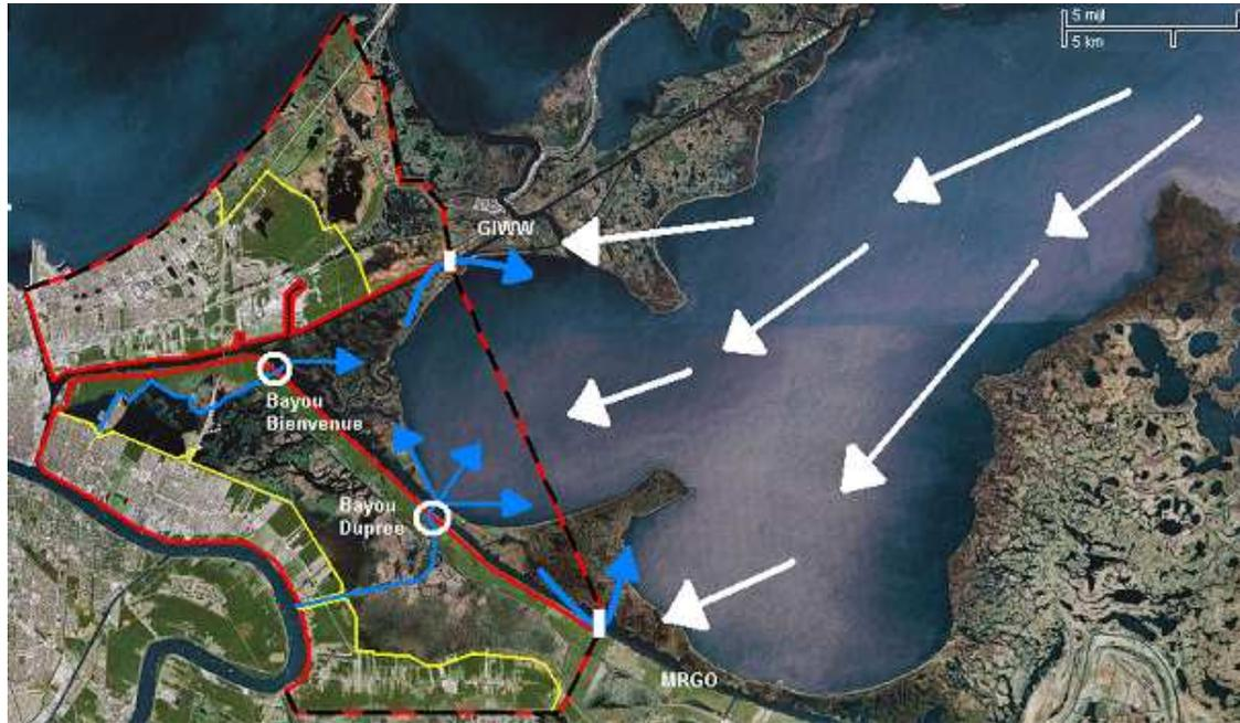
Fig. 4.7: Retention area for flood protection, retention of rainfall runoff and preservation of wetlands
