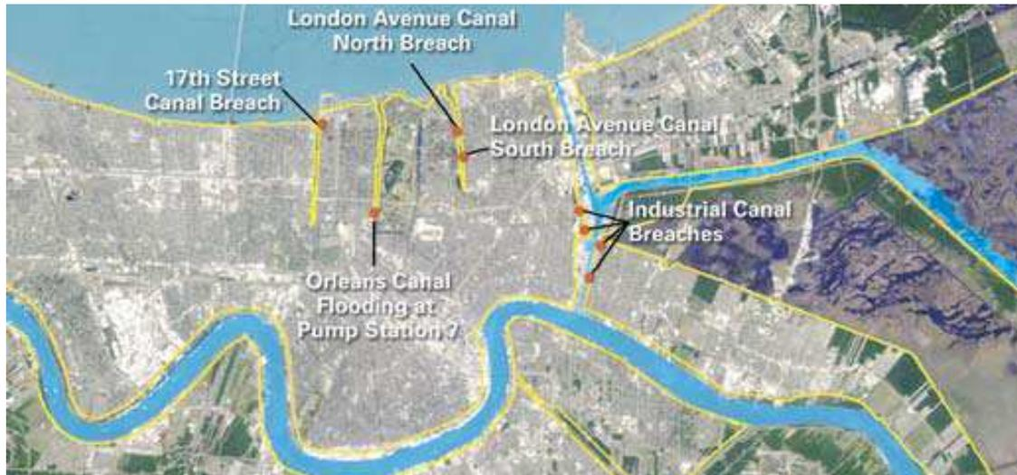
Fig. C.4: Overview of the failures of several I-walls and levees along the canals into New Orleans [1]
