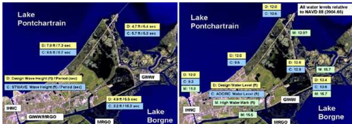
Fig. 4.2: Orleans East Parish: comparison of wave maxima (left) and water level maxima (right) with design values
