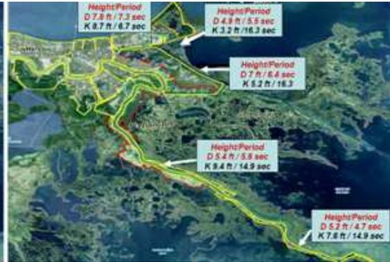
Fig. 1.10: Comparison actual wave conditions with design [29]
