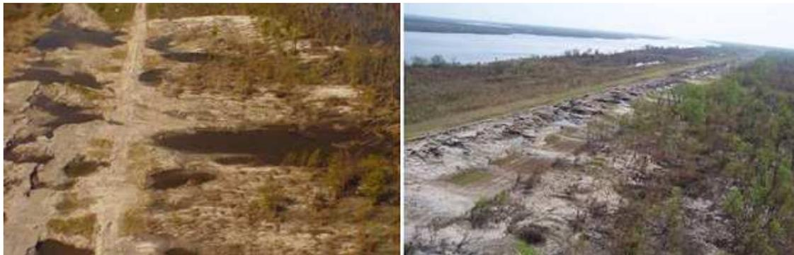
Fig. 3.7: Examples of levee breach along the GIWW (left) and the MRGO (right) [29]
