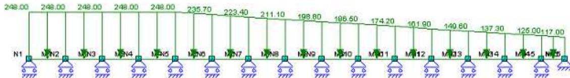
Fig. 8.13: Model front plate and schematized loading
