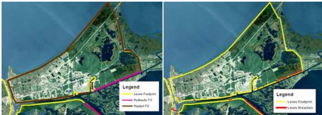
Fig. 3.8: Levees along the GIWW / MRGO – correlation between erosion and types of material used [32]
