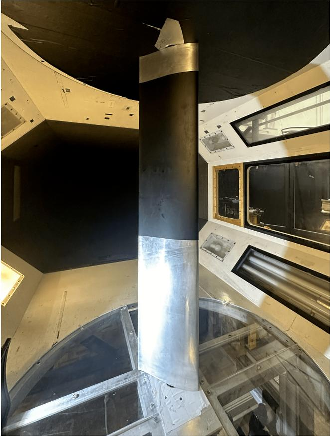
Figure 3.2: NACA643418 airfoil within the wind tunnel, depicted at a 50° angle of attack.
