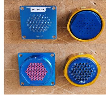
(b) Connectors designed for interfacing the pressure tubes with the pressure reading device.<sup>1</sup>
