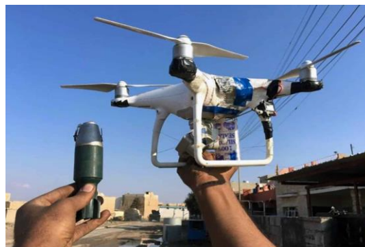
Figure 1: Modified drone carrying a grenade [4].
