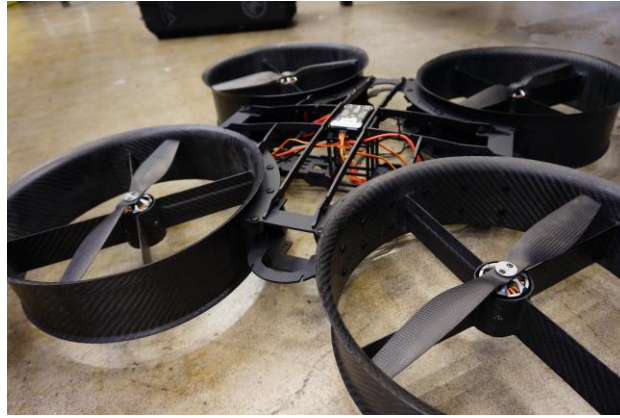
Figure 16: Ducted fan design drone [38]. The blades are covered by conducting materials and the micro-Doppler effect is not examined.
