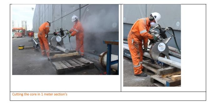
After cutting the cores the cores were further processed by the TU Delft Team. They additionally labelled and photographed the core ends, foaming (by IOT), cap & clipping, packing into the core transport box container and transporting the cores to the TU Delft facility.
