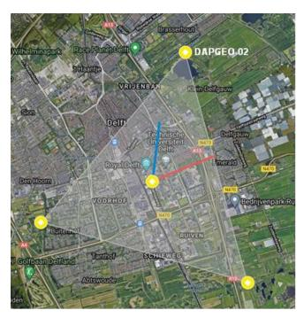
Figure 4. Local seismic monitoring network (yellow circles) around the campus geothermal wells (base map source: google maps).
