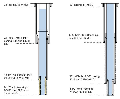
Figure 8. Well schematics of DEL-GT-01-producer (right) and DEL-GT-02-S2-injector (left)
