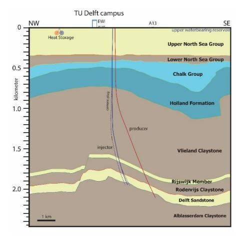
Figure 7. Schematic illustration of the producer and injector trajectories at depth. The dotted lines are the two sidetracks DEL-GT-02-S1 and DEL-GT-02-S2, respectively.
