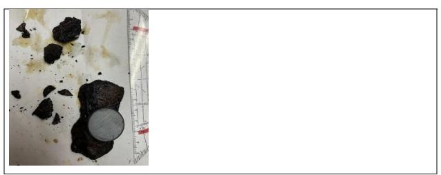
Corroded metal found on top of the ball (activations sub)
