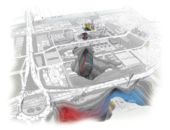
Figure 1: Illustration of the Campus geothermal project, including the currently gas-fired power plant, the heating grid, and the geothermal doublet (illustration credit: Total shot productions).
