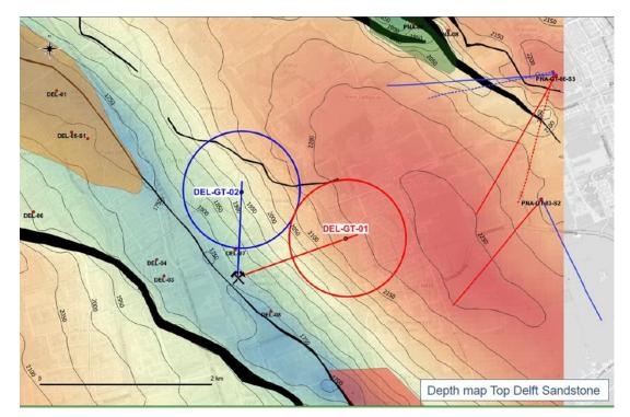
Figure 3. Location of the campus geothermal project (producer and injector; DEL-GT-01 and DEL-GT-02) at depth. Also included are two other geothermal project targeting the same reservoir (source GTD).
