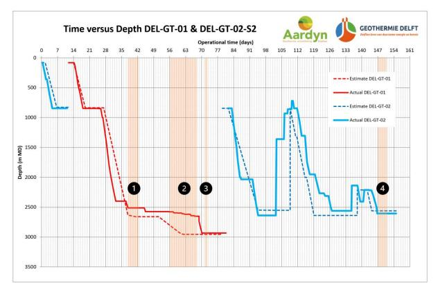
Figure 9. Time vs depth both wells (GTD) The marked orange areas indicate research activities. These have been marked with numbers (1) core #1; (2) core #2-7; (3) open-hole logging 3 runs and (4) open hole logging 3 runs + side-wall coring 3 runs.
