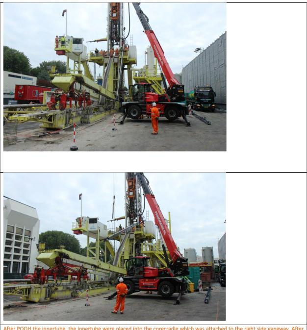
After POOH the innertube, the innertube were placed into the corecradle which was attached to the right side gangway. After this was done, the Manitou could gently lift the corecradle into a horizontal position and place the corecradly at the processing area.
