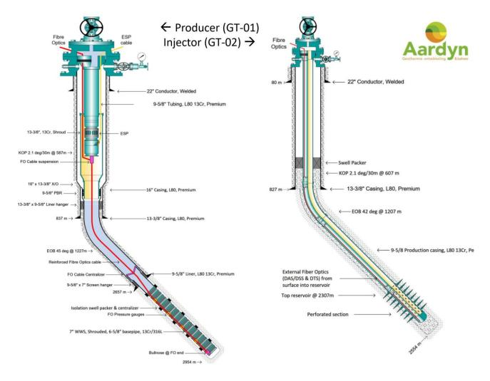
Figure 5. Pre-drilling well designs including R&D components of the Producer (DEL-GT-01) and the Injector (DEL-GT-02) wells drilled at TU Delft campus (source GTD).
