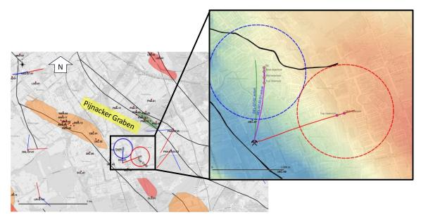
Figure 6. Producer (DEL-GT-01 in red) and injector (DEL-GT-02 in blue) location within the Pijnacker Graben. Zoom shows doublet as installed and including sidetracks; DEL-GT-02 in green, DEL-GT-02-S1 in purple, and DEL-GT-02-S2 in blue (source GTD).
