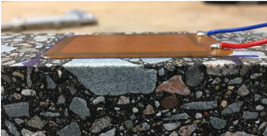
(a) Closeup of Sensor attached firmly to asphalt
