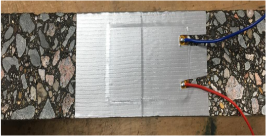
(b) Sensor fixed to asphalt and duct taped leaving electrical contacts open
