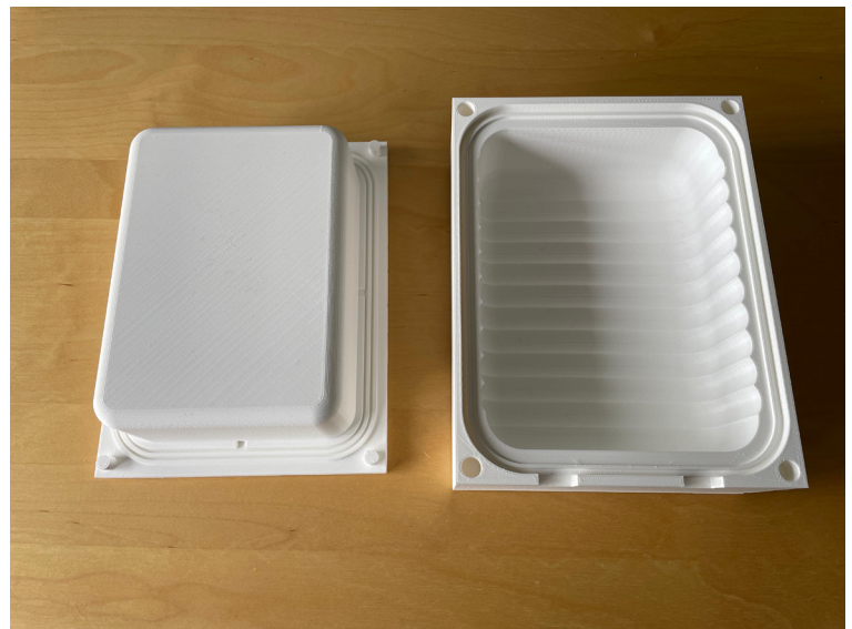
Figure 38: FDM 3D printing of silicone mould
