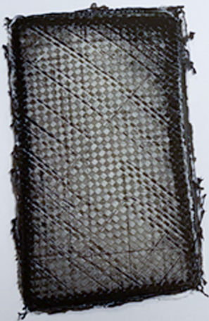
Figure 56: Bending test samples of 170 °C with the following orientations: a) 0/45, b) 45/0, c) 0.
