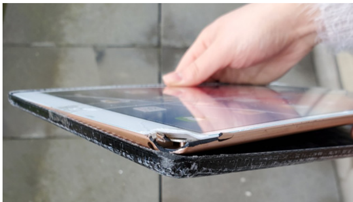
Figure 98: Damage on dummy iPad after alternative drops.
