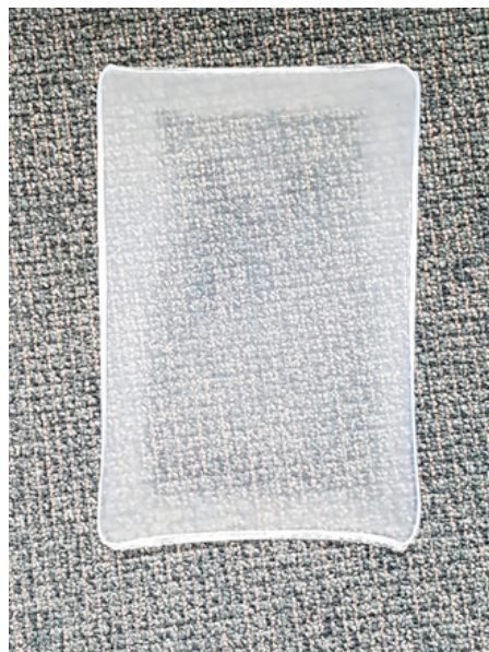
Figure 71: PP laminate with transparent and matte areas.
